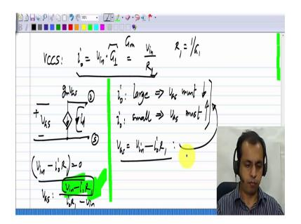
Now, a voltage controlled current source follows the relationship  $i_o = v_{in}G_1$ . This is usually denoted by  $G_m$ , but do not confuse between  $g_m$  of the MOS transistor and this  $G_m$ , I will use a
