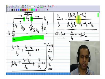
Let me copy over this. Now, I will write the equation at this node, and the equation at that node, that is the total current flowing into that node, current flowing in  $R_s$  is  $(V_s - V_{GS})/R_s$ ; by the way, this  $V_{GS}$  is also measured with respect to ground, because this source is grounded, so, be careful about that, that may not be true in all circuits; plus
