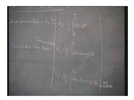
It is easier to remember these as saying a nought equals the average value of f of t. Whenever, I am talking about average, it is average over 1 complete period and a n is 2 times the average value of the product f of t cos n omega nought t and likewise b n is 2 times the average value of f of t sine n omega nought t. So, these are the 3 integrals that 1 makes use of to evaluate the various Fourier coefficients.
