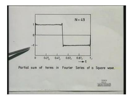
So, you can see as you go on increasing the terms then the series the truncated series approach is the original f of t very closely, i would like to show another figure which shows how different harmonic components add up to build a composite wave.
