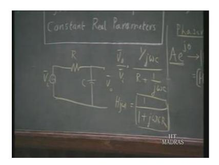
So, analysis of systems with of the type that is; described here under sinusoidal excitation becomes almost a kind of mechanical procedure algebraic procedure instead of our having to deal with differential equations. The fact that a system with arbitrary complexity involving a differential equation of high order can be analyzed in a purely algebraic fashion as here constitutes the central advantage of the phasor concept and the simplicity of a c circuit analysis methods.
