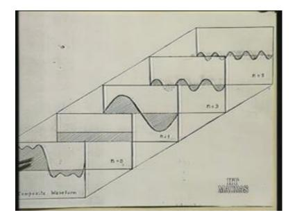
Suppose, this is a composite wave form that, we would like to have in this case there is d c term there's a fundamental there's a third harmonic and there's a fifth harmonic. The composite wave that, i have drawn here is 1 which is built from this. Therefore it really means that; there is only 4 terms in this Fourier Series expansion and the 4 terms in the
