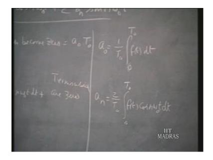
So, b n will be 2 up on t nought 0 to t nought f of t sine n omega nought t d t. So, these are 3 formulas which can be used to evaluate these various integrals.
