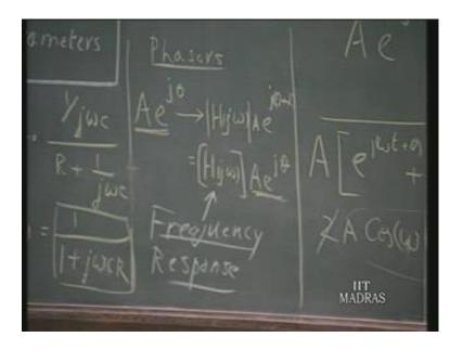
So, this is a very convenient 1 and we would like to make use of this facility to the extent that is possible and what is meant by frequency response function. It is the ratio of the output phasor to the input phasor under steady state sinusoidal conditions. However, in practice in real systems we may not always have excitation functions which are
