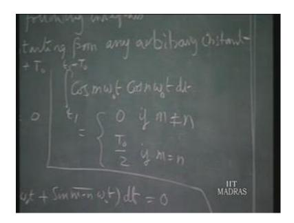
So, these are the background results we need for setting up formulas for evaluating the Fourier coefficients you recall that, the formula for we said that, f of t can be expanded as a nought plus a n cos n omega nought t plus b n sine n omega nought t suppose, you
