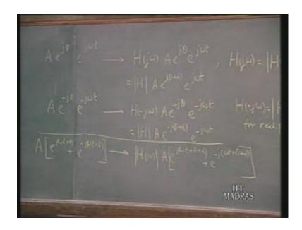
That means this is a general sinusoidal function of time and as far as the output is concerned you have h j omega magnitude 2 a cos omega t plus theta plus alpha. So, what do we have we have a sinusoidal function of time with an amplitude 2 a. The output is modified is also a sinusoidal function, but the output is magnified in magnitude by the this factor magnitude of the h of s which we call the system function as we recall.
