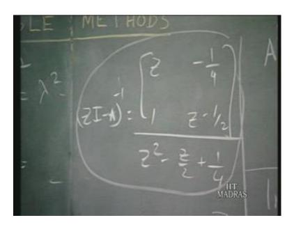
So, this after simplify you get Z squared plus Z divided by Z squared minus Z by 2 plus 1 fourth. That then is the transfer function you can also obtain this transfer function as an alternative by taking the Z transform of this. The Z transform of the impulse response must be the transfer function. So, hence you know the impulse response you can take the Z transform of that. Because, the same result but, what we have done is we are derived it directly from the formula both are equal.
