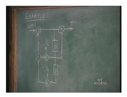
So, to set up this state and output equation we will consider the state variables to though which are at the outputs of the delay units. So, we will call that X 1 n the signal here X 1 n will call the signal here X 2 n. So, once you are identified the 2 state variables then the state equations can be written X 1 n plus 1 and X 2 n plus 1 equals half minus 1 quarter 1 0 X 1 n and X 2 n. We can easily see that X 2 plus 1 is X 1 of n itself. So, X 2 n plus 1 is
