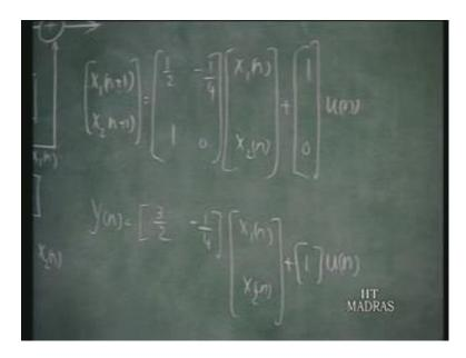
That is the this at the state and output equation for the systems. Now, we would like to find out the state transition matrix for this. So, lambda I minus A determinant equals 0 it turns out this will be equal to lambda squared minus lambda by 2 plus 1 quarter equals z0. This is the characteristic equation. So, the 2 characteristic values lambda 1 and lambda 2 can be shown to be half e to the power of plus or minus j pi upon 3.
