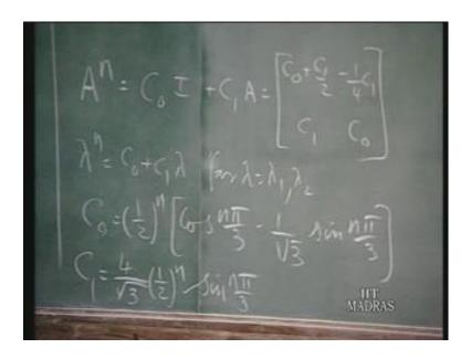
Therefore, you substitute C not and C 1 into An you get the state transition matrix An it turns out ot be half raised to the power of n cos n pi upon 3 plus 1 by root 3 sin n pi upon 3 1 by root 3 sin n pi upon 3 minus 1 by root 3 sin n pi upon 3 and here cos n pi by 3 minus 1 by root 3 sin n pi by 3. That then is the state transition matrix.
