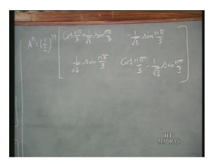
Now, suppose I want to find the impulse response hn. It is as we already observed this is equal to D for n equals 0 and C A n minus 1 B for n greater than or equal to 1. So, using the value of An so that means instead of n you must put A n minus 1 substitute over here
