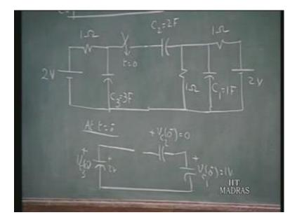
Now, at t equals 0 plus you have again the switch is closed therefore, these 3 capacitors form a loop v c 1 0 plus. And let us say this is v c 2, this is the reference sign we have taken v c 2 0 plus and this is v c 3 0 plus. So, we have a new regime at t equals 0 plus v c 3 0 plus v c 2 0 plus and v c 1 0 plus. Kirchhoff's voltage law tells us v c 3 0 plus equals v c 1 0 plus plus v c 2 0 plus right. But what is v c 3 0 minus 2 volts? V c 3 0 plus may be not be 2 volts.
