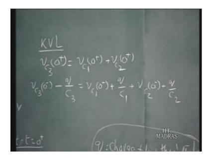
That turns out to be if you solve this you will have let me write this down here: q times 1 over c 1 plus 1 over c 2 plus 1 over c 3 solving this equation you will get this as 1. That is the balance the unbalanced voltages that we get here and from we get q equals 6 by eleven coulombs. And therefore, you have v c 3 0 plus we can calculate using this.
