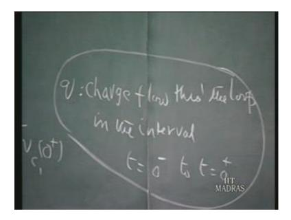
D q by d t will turn out to be impulse the current is impulse, but the area under the impulse is finite. Therefore, instantaneously an additional charge must flow and what is the value of this charge v c 3 0 plus equals v c 3 0 minus this is v c 3 0 minus, And there is a charge q coming out therefore, the resulting voltage drop is q by c three.
