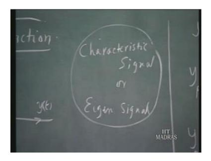
Again, the meaning of an eigen signal or a characteristic signal is it is that particular signal which if it is given as input. The output will also will have the same time variation except for a scale factor and that scale factor is h of s in this case. So, e to the power of s t is a characteristic signal e to the power of s t with a constant multiplier any constant is a characteristic signal of linear time invariant continuous time systems. This is a very important property.
