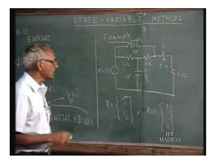
For this purpose we take the same example that we have used while illustrating the Laplace transform technique. So, the example that we take is we have a switch here which is closed at t equals 0. And we have an inductance at this point. Now, the driving source is a 1 volt dc source. This is 1 ohm, this is 1 farad, this is 1 henry, this is 1 ohm and this is 1 ohm. We take the state variable to be il and vc is a form the natural choice.
