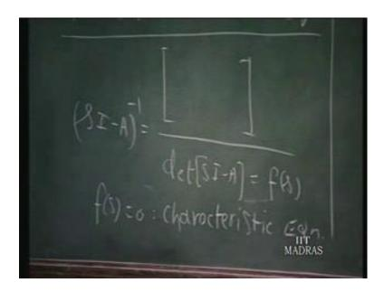
Is a square matrix of order n. If, I take the inverse of that you will have, a matrix which corresponding to a joint of this divided by the determinant of sI minus A. The determinant of sI minus A as you can see is a polynomial in s. Because, A is a matrix with constant coefficient and therefore, there is s only the diagonal terms. So, if you evaluate the determinant you will have a polynomial in s of degree n where, n is the dimension of the state vector.
