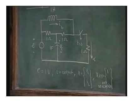
A voltage source e let us take this e to be 1 volt dc. That forms the input quantity single input and i is the output, this is the output. We have 1 inductor and 1 capacitor, we take V c and i L as the state vector v c and i L. So, we have this is correspond to u. This corresponds to Y and this corresponds to this state vector. We close the switch at t equals 0 and we are asked to find the solution for i.
