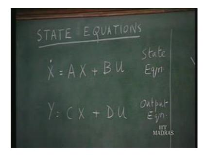
The X dot equals AX plus Bu which called the state equation. Y equals CX plus Du the output equation. These are in time domain. Collectively they will call state equations; even though this particular matrix equation is referred to discrete equation. Now, this is a, these 2 equations are actually matrix equations where, each matrix is have an appropriate dimensions X X dot u and Y are columns or vectors. A B C D are matrices appropriate dimensions.
