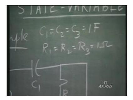
To simplify numerical work let us take C 1 equals C 2 equals C 3 equals 1 farad. And R 1 equals R 2 equals R 3 equals 1 ohm. Now, we observed that the 3 capacitors and the 2 sources form a loop consequently the sum of the capacitor voltages and the sources must add up to 0 by according to kirchoff's voltage law; which means; that 3 capacitor
