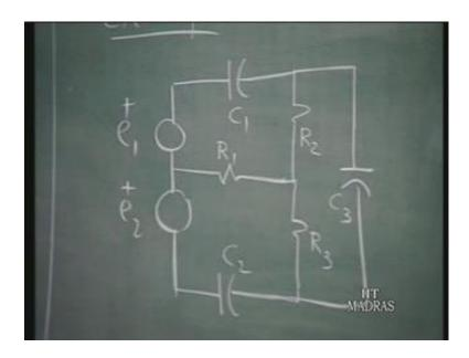
Let us consider that we have a circuit in which 2 sources are acting we have 3 resistors and 3 capacitors like this. So, let this is C 1 this is C 2 and this is C 3. And this is R 1 R 2 and R 3.
