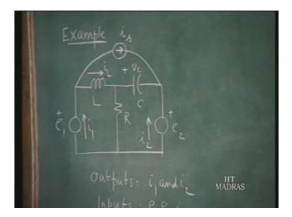
Let us consider: a network like this containing an inductor a resistor and capacitor and there are 3 sources e 1 e 2 voltage sources and a current source i s. So, this is an example how various representative elements 1 resistor, 1 inductor, 1 capacitor 2 voltage sources and current source. So, the input quantities are e 1 e 2 and i s time varying quantities that the sources. And we decide to find the solution for i 1 and i 2. So, i 1 and i 2 are the output quantities of the responses.
