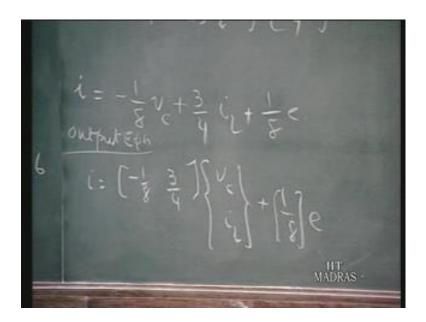
Therefore, i equals 1 fourth Vc dot that means minus 1 by 8 Vc plus 3 upon 4 times iL plus 1 by 8 e or to put this in the standard matrix form i equals minus 1 8 3 quarters Vc iL plus 1 eighth e. So, in this this is the output equation, in the standard form.
