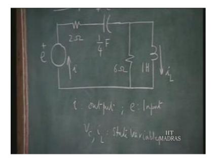
Let us, consider this example in which we have a capacitor and inductor. Let us, assume that this particular circuit is excited by a voltage source e and we are interested in finding out I as the output quantity. That means, our output vector 1 y consist of just 1 variable that is i. And let us take Vc the capacitor voltage and inductor current iL as a state variables.
