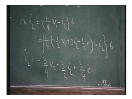
The voltage across this inductor is L di dt so, 1 times iL dot that is the voltage across the inductor. And that voltage is also equal to this voltage which is 1 fourth Vc dot minus iL times 6. And Vc dot is known to us already therefore, 1 fourth of for Vc dot is substitute minus half Vc plus 3 iL plus half e. That is Vc dot which we already known minus iL and the whole thing multiplied by 6.
