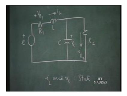
Suppose, we have a network of this 1 inductor and 1 capacitor and 2 resistances R1 and R2. Let us, say we are interested in these 2 values VR1 and iR2. These are the 2 output quantities, which we are interested this is the input excitation. So, in order to solve this particular circuit even the value of E from say t equals 0 onwards. The solution can be unique only if you know, the initial value of the inductor current and capacitor voltage.
