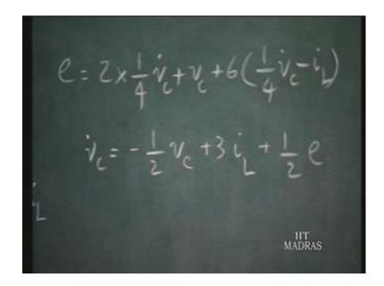
Therefore, I can write e is 2 times this is 2 times the current in that 1 fourth Vc dot plus that is the voltage across this drop, voltage drop across the resistance plus this voltage which is Vc plus the voltage drop across 6 ohm resistor which is 6 times the current through this 1 fourth Vc dot minus iL. And that if you simplify this you will get, Vc dot equals minus half Vc plus 3 iL plus half e this is 1 equation. Similarly, we must also have the equation involving iL dot.
