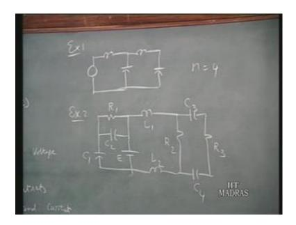
Second example, suppose I have this call this C1 C2 E R1 L1 L2 R2 C3 C4 R3. Now, in steadly quietly complicated situation, you observe that there is a loop here constitute by C1 C2 and E. So, if I know some voltage across the capacitance I know the voltage E therefore, this capacitance voltage gets fixed. Therefore, you cannot arbitrarily assign in the initial condition for both C1 and C2 only 1 of them you can independent you can assign.
