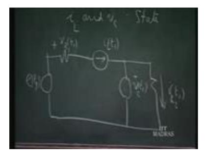
As seen in this example, the state is described by a set of dynamically independent variables iL and Vc in this particular case.
