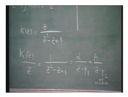
So, to do the partial fraction expansion of this, we will first of all divide right through by z according to our practice. So, z squared minus z plus 1. That we say this is equal to alpha over z minus p 1 plus beta over z minus p 2, where p 1 and p 2 are the poles of this reactional function.
