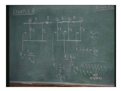
Let us now consider as a second example, a ladder network which has a value of all resistors equal to R 1s in this configurations. Let us say at this is 1 end of the ladder. So, the effective resistor is seeing here I will call that R 1. So, look in to it right, what is the effective resistance still at this point is R 1. Now, the second step, say let us say this is node 1, this is node 2, this is node 3 and there are all nodes let us say N nodes, this are the node names.
