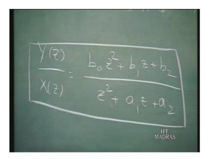
We have Y z over X z equals b not z squared plus b 1 z plus b 2 divided by z squared plus a 1 z plus a 2. So, we now have instead of difference equation connecting y n and x n in the transform domain, we have a pure raised your Y z over X z is b not z squared
