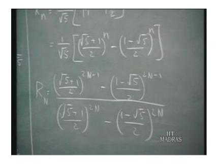
And the R N that we are looking for, the effective resistance seen at this end at the N'th node, which is K 2 N minus 1 by K 2 N, it now can be written as divided by root 5 plus 1 by 2 raised to the power of 2 N minus 1 minus root 5 by 2 raised to the power of 2 N. That is being expression for R N. So, we can find out the effective resistance for general value of N using this particular expression.
