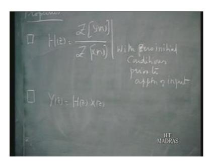
What are the properties of the system function? First: H of z is that we repeat this Z transform of output quantity by the Z transform of the input quantity, with 0 initial condition prior to the application of input, it obvious. That is the definition. Second point of course, with 0 initial condition once again Y z equals H of z times X of z. This is just repeating, but putting in alternative fashion.
