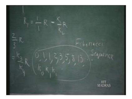
And by the way, such sequence of numbers, where each number is the sum of the proof receding number is known as Fibonacci sequence or Fibonacci numbers Fibonacci sequence of numbers. And interestingly in ladder network, with all equal resistances then the effective resistances at any particular node can react in terms of the Fibonacci sequence numbers. But, we would like to find out a general expression for K n; that is the problem that we have 1 hand.
