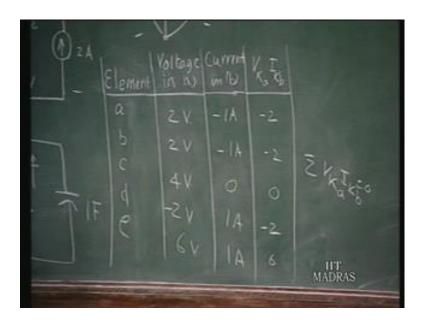
Now, you observe that as far as element d is concerned, this is positive with reference to this, but this is positive with reference to this therefore, you must write this as minus 2 volts. So, if you add up all these sigma V K a I K b is 0. So, the sum of all this impedance is 0. This is just an illustration of Tellegen's theorem, applicable to 2 networks with identical topology, but different elements.
