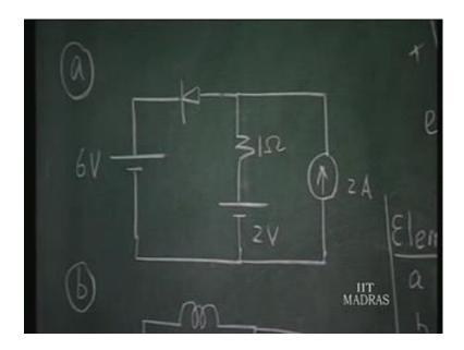
Suppose you open circuited this point, then this 2 amperes goes through this so, developing a 2 volts here 2 volts here therefore, this 4 volts developed across this and this is 6 volts. That means the diode is reverse biased and therefore, it does not conduct. Therefore, the voltages in first network can be obtained.
