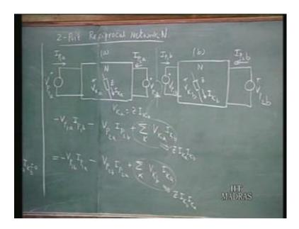
Let us consider the same network containing reciprocal elements under 2 different excitation conditions. So, this is under condition a, this is under condition b. So, I put V p 1 a, that is, port voltage 1 under network a condition a and the corresponding current I p 1 a, this is V p 2 port p 2 means port 2 a and the corresponding current I p 2 a. And there is general elements here inside the network; let us say impedance z. It has got a voltage V K a and a current I K a.
