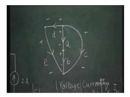
Now, we would like to illustrate the Tellegen's theorem here with respect to this network, taking the voltages in network a and currents in network b. So, if you find the voltages in network a, what happens is; when what is the diode conducting or not.
