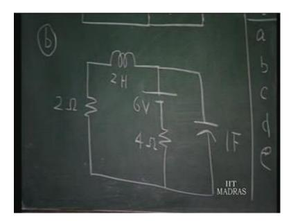
And similarly as far the current network is concerned, second network is concerned it is a DC network. We want to illustrate this under steady state conditions. The capacitor is open circuited therefore, this 6 volts drives a current through this loop and this current will be 1 amperes because, 6 volts divided by 6 ohms is 1 ampere. And as far as this is concerned the under steady state conditions 2 volts is developed here and the voltage across this is 2 volts.
