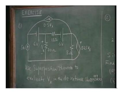
Problem number 1: we have essentially a DC network, in which there are 2 independent 3 independent sources; 2 voltage source and a 1 current source and we have 2 dependent sources; 1 voltage source and a current source both dependent on the control voltage V x. So, you take down this particular figure and use superposition theorem to evaluate V x in the DC network shown.
