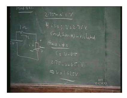
You have the Thevenin's equivalent as far the terminals are concerned, you have 2.75 volts and Thevenin's resistance is 1 ohm. And this is now connected to the non-linear resistance here, which has got this V i relation. So, you can say that, you can solve this problem using the load line approach which you are familiar with electronic circuits or alternately you can do it analytically. If this is current is i 2.75 minus i times 1 minus i; that is the voltage across this a non-linear el element.
