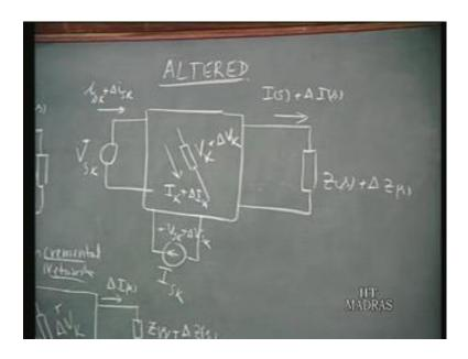
In this altered network, we have the same voltage sources and current sources. Same elements inside but, one particular impedance Z s is changed to Z s plus delta Z s. Consequently, all the values except the strength of the independent sources will be realtered. The current in this originally was I s, may altered as I s plus delta I s. The voltage here may be altered from V k plus delta V k, I k current I k plus delta I k.
