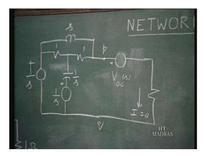
I would like to see what happens, when the switch is closed. This is what we are having. When switch is closed, you want to find out the current here, I of s. Now, let me introduce here 2 voltage sources. Let me say, when switch is open. Suppose, when the switch is open the voltage across this, which is V o c t. After all, that is the open circuit voltage. And let its Laplace transform be V o c of s.
