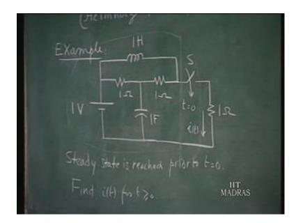
Let us now consider this example, as an illustration of the application of the Thevenin's theorem. We have in this circuit, two resistances one capacitor and one inductor. All of unit value, with a 1 volt source. The switch is kept open for a long time, still steady state is established. And it is then closed, at t equals 0. We are interest in finding out the current i t. So, to solve this problem there are several approaches, of course.
