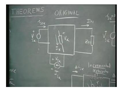
To introduce the compensation theorem, let us consider this network. This box contains linear elements. It is acted upon by several voltage sources, I represented one of them called V s k. Several current sources, the kth current source is represented here carrying a current I s k. The current produced by the voltage source, I call I s k. Just to distinguish between this and this, I use the lower case letters here.
