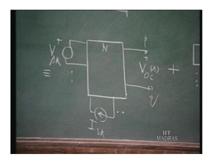
In the first network, I still keep this linear network. But, it is acted upon by the original voltage sources, that are present in N A. And the current sources that are present in N A. But, this I L of s is deactivated. So, that is kept open circuited. So, the two terminals are kept open circuited. And let as a result of this, we have a voltage V o c of s developed across p q. This is called the open circuit voltage.
