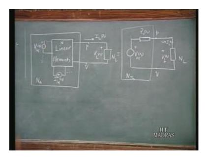
Our discussion so far, has told us that a network like this, with N containing linear elements plus acted upon by several sources. It can be replaced by an equivalent circuit of this type, where there is one source which has a voltage which is equal to the voltage across the open terminals of p q. When N L is disconnected, that is called the open circuit voltage. And in series with an impedance, which is the impedance measured.
