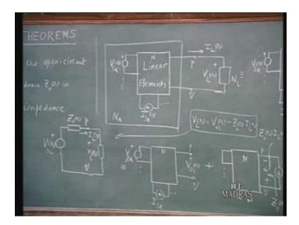
That is the exactly, what this equation states. Therefore, for any given I L of s, V L of s will be given by this equation. This will also be given by this equivalent circuit. And that is what constitutes the conditions in the original network. After all for a given I L of s, V
