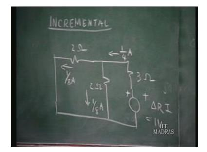
So, you have delta times original current 1 volt. Change is 1 ohm. Current is 1 ampere. Therefore, this is a source of 1 volt. A DC source acting in a circuit, in which the original sources are deactivated. So, these 6 volts is deactivated. It is replaced by a short circuit. So, if you analyze the circuit which consists of 3 ohms and 2 2 ohms in parallel. The currents will be one fourth ampere one eighth ampere and one eighth ampere.
