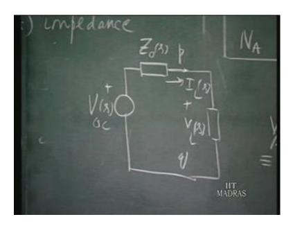
If I have a voltage source V o c of s, in series with a one port whose impedance function is Z naught of s. And I say, these are the terminals p q and whatever I connect here. If this is current is I L of s and the voltage is V L of s. So, V L of s equals V o c of s minus Z naught of s times I L of s.
