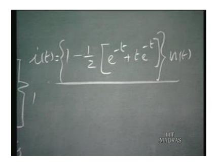
That is 1 minus half e to the power of minus t. From this, you get t times e to the power of minus t the whole thing of n of t. That is the current. 1 minus half e to the power of minus t minus half t into e to power of minus t. That is the solution for this. Now, I would also like to demonstrate the use of substitution theorem, to get the same solution. Now, let us look at this.
