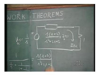
So, the up short of all this analysis therefore, is Thevenin's equivalent as 1 over s as the open circuit voltage. And a one port network, whose driving point impedance is s times s plus 2 over s square plus 2 s plus 2. This is equal to Z naught of s. This is the Thevenin's
