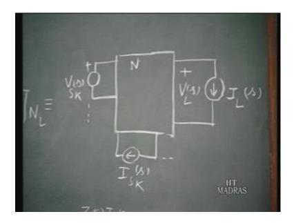
Now, I would like to calculate this V L of s in this network, by superposing the effects of because of, n is linear and we have several source acting on them. So, n is linear network. And this linear network is acted upon by several voltage sources, several current sources I s k of s L plus a another volt source, current source I L of s. So, in order to calculate V L of s, I take up the approach of superposition.
