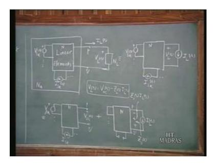
Therefore, the voltage that is developed across the terminals p q is minus Z naught of s times I L of s, if you take p positive. And Z naught of s times I L of s, if you take q as positive. Anyway, the overall V L of s therefore, after all the sum of these two must be equal to this one this voltage, which is equal to this voltage of course. So, as a result of this we get V L of s equals superposing these two effects.
