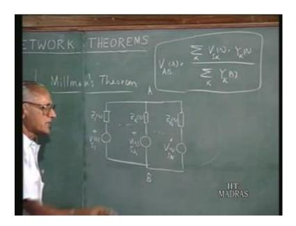
I would also like to mention in this context an extension of these results, which go by the name Millmans's theorem. These are all the straight forward extensions of this, same similar concepts. Millman's theorem is applicable to a parallel connection of several sources. So, V s s 1 of s Z 1 of s. Suppose, you have whole series of such branches and I will say, this is the kth branch V s k of s Z k of s. And like that, let us say that a last branch is Z n of s and V s n of s.
