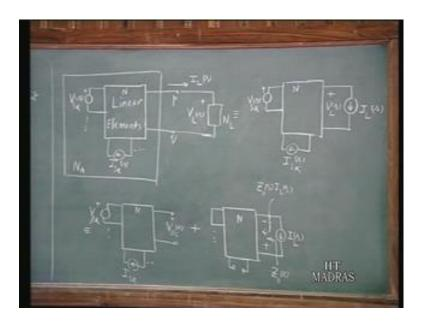
So, if I connect I L of s a current source of exactly as same magnitude as this, same value as this same function as this then, there should not be any disturbance created in the network. So, all elements will continue to have the same variables associated with them. So, if I connect a current source here, replace this N L by a current source as I should. I should still get V L of s here. And all elements inside, must have the same variable associated with them.
