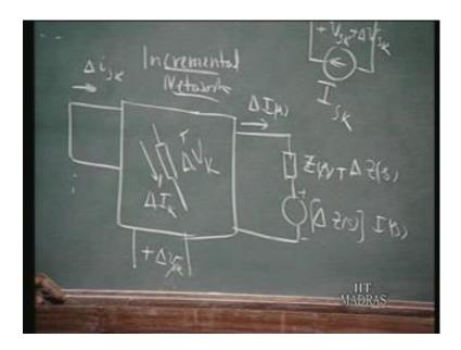
The compensation theorem tells us, you consider this network in which all the independent sources are deactivated. So, the voltage sources are also replaced by short circuit. The current sources are open circuited. In this are internal elements. So, the original current impedance Z l is carrying a current I s. So, you have a voltage source whose strength is delta Z s, the change in the impedance times the original current.
