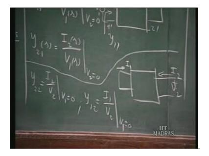
Now, suppose I want to find out y 1 2 of s and y 2 2 of s. So, y 2 2 I will drop the functional notation s within brackets to simplify my writing y 2 2 is I 2 by V 2, when V 1 is 0. So, I 2 by V 2 at V 1 0; that means, the experiment that you suggested is in this 2 port network you short circuit this and you apply a certain voltage V 2 and measure I 2 the ratio of these two is Y 2 2 of s.
