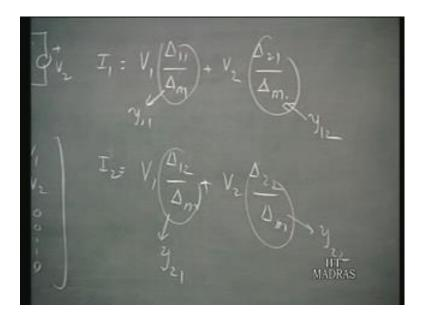
So, from this you can calculate I 1 and I 2 by taking the ratio of the appropriate determinants. And if you do that you will get what I 1 equals V 1 times delta 1 1 by delta m, where delta m is the mesh based a system determinant and delta 1 1 is the co factor plus V 2 times delta 2 1 by delta m. That is you replace the when you calculating I 1 you replace that in first column by this column V 1 V 2 and 0 and when you expand that you will get this.
