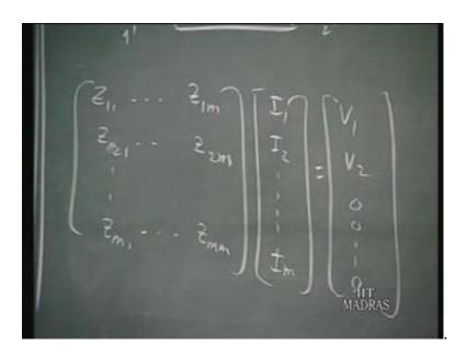
So, you can write the loop equations of this network, we have say Z 1 1 say there are m loops Z 2 1 Z 2 m Z m 1 Z m m. These are the loop equation I 1 I 2 I m as far as the forcing function is concerned, you have the sources only in this loop quadrants two. Because internally, it is suppose to be a passive network linear time invariant network no independent source are present. Therefore, we have V 1 of s and V 2 of s here for the second loop all the others are 0s.
