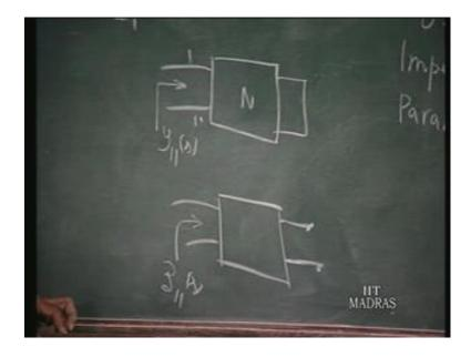
Look at the definition of Y 1 1, how do you define Y 1 1 is the ratio of I 1 to V 1 when V 2 is 0. So, you short circuit this and measure this admittance and that is y 1 1 of s, how do you define z 1 1 it is the ratio of V 1 to I 1 when I 2 is 0, so the you are keeping this open circuit at. And measuring these impedance that is z 1 1 of s. So, the network in which this admittance is measured and the networks in which this impedance are measured are different.
