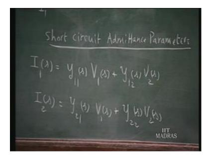
Here, we treat I 1 and I 2 as the response quantities and V 1 and V 2 as the input quantities. So, I 1 of s is linearly related to 2 the input quantities V 1 and V 2 and the proportionality constants for that are written as y 1 of y 1 1 of s times V 1 of s plus y 1 2 of s times V 2 of s. So, the response in this the response of current I 1 is really related to the input quantities V 1 and V 2 by the proportionality constants y 1 of s and y 1 2 of s.
