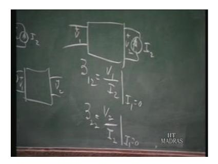
Therefore, you should make I 1 0 and introduce a current I 2 here. And this is the response V 2 and this is response V 1 z 1 2 is V 1 divided by I 2. When I 1 is 0 and z 2 2 is V 2 divided by I 2 when I 1 is 0. So, these definitions are completely in parallel with it defining relationship for the y parameters except now the currents are the excitations sources.
