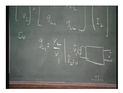
And once again, you can define example if I want to find out what g 2 1 is is V 2 over V 1 when I 2 is 0. Because, V 2 is g 2 V 1 plus g 2 2 I 2, therefore when make I 2 equal to 0, V 2 equal g 2 1 times V 2. So like this, you should be able to define each one of these parameters with the appropriate terminal conditions.
