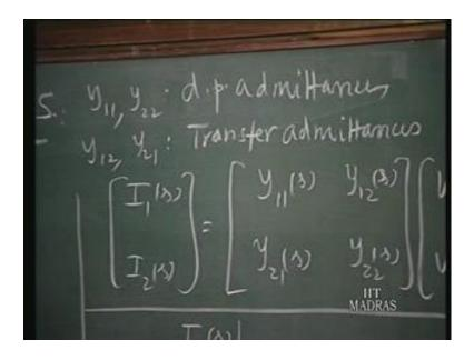
Now, y 1 1 and y 2 2 are called driving point in admittances y 1 1 and y 2 2 are the driving point admittances, because the response. And the input at the same location associate the same terminal pair either in the case of y 1 1 or in the case of y 2 2 I 2 or V 2.
