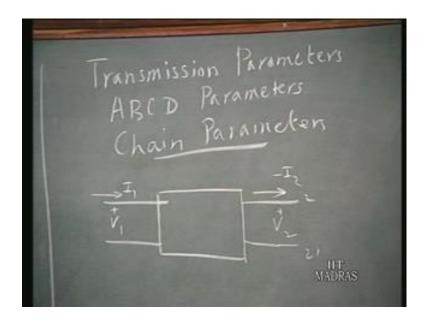
In addition you also have another important category of parameters which go by the name transmission parameters also called ABCD parameters sometimes called chain parameters. Here, assume that this is the transmission line and you are talking about the output of the transmission line. This current is minus I 2, because we are we are defining the port I 2 as leading inwards. Therefore, 2 2 prime this the voltage and current that is being fed from the at the output end.
