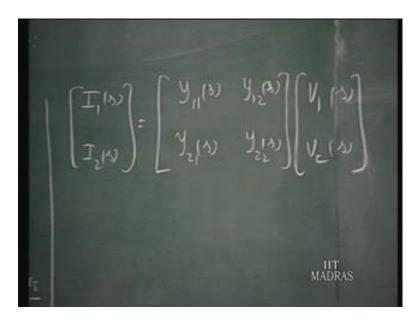
In matrix form the same set can be written in very convenient fashion I 1 of s I 2 of s is obtained as the y 1 1 of s y 1 2 of s y 2 1 of s y 2 2 of s multiply it V 1 of s V 2 of s. So that is the convenient way in writing down the parameters in matrix form relating the currents to voltages.
