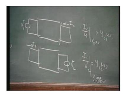
As an obvious of this, what we have here is? Suppose I have 2 port network and let us say this is the raw form of the network. This is a basic network, if I introduce a voltage source here, V 1 and measure the current here I 2. So, this is I I 2 by V 1 when V 2 is 0, this we call this as y 2 1 of s we know that.
