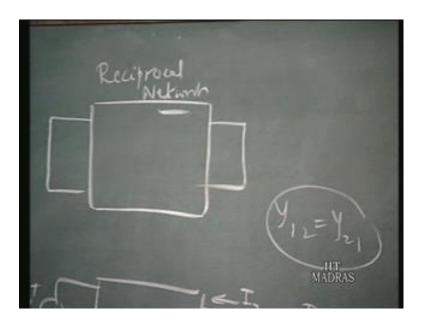
Now in this raw form of the network, suppose I introduce a voltage here V 2 and measure the current response here I 1. Then, I 1 by V 2 is y 1 2 of s, this is what we say when V 1 is 0, this 1 how we define. So, if this is reciprocal network y 1 2 must be the
