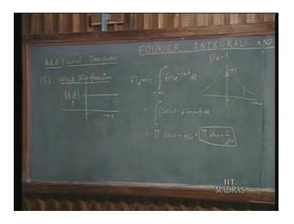
To start with, let us take the unit step function u of t. This of course, has a value 1 for positive t and 0 for negative t u of t is the unit step function in the sense. Now, 1 we like to find out the Fourier Transform for this. So, F of j omega 1 over 2 pi integral from minus infinity to plus infinity of f of t e to the power of minus j
