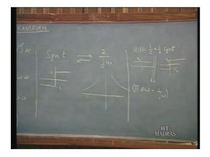
Therefore, this will become minus 2j over omega or I can write this as 2 over j omega. So, the absort of this now, to say that the signum function of t minus 1 plus 1 that is, signum function of t has its Fourier Transform 2 upon j omega. And therefore, when we had in the derivation of the unit step function, you recall that once again that let me redo what we done there.
