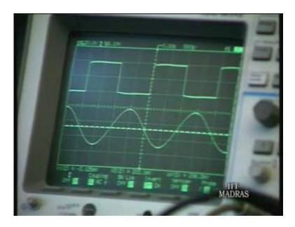
You, observe that the output of the low pass filter corresponds only, the fundamental a pure sine wave. And this has the amplitude which is about 4 upon 5 times the amplitude and square wave as we should expect. Now this is the, that is the only the fundamental is pass through. Now, if you allow other frequencies for example, if increase the cut off
