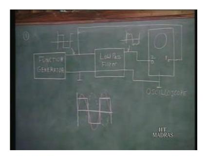
Demonstration we have just now witnessed in the first part of the experiment. You had a function generator which produces the square wave. This is put through low pass filter which allows frequencies up to certain order to pass through. And both these square wave and output of the low pass filter are displayed on the oscilloscope. oscilloscope has 2 channel 1 channel you have the square wave and the channel below we displayed this type of wave form.
