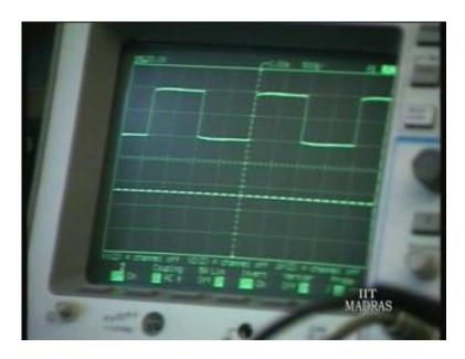
So, let us see what we have here, is a 500 square wave. And now, I am putting a low pass filter cut off frequencies. So, that only the fundamental pass through and when you do that.
