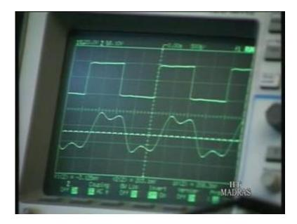
Is also coming through and we can increase the cut off frequency and allow more and more harmonic come through. And as you can see, as you pick up more and more harmonics the output becomes closers to the square wave. In fact, if you go to very cut off frequency.
