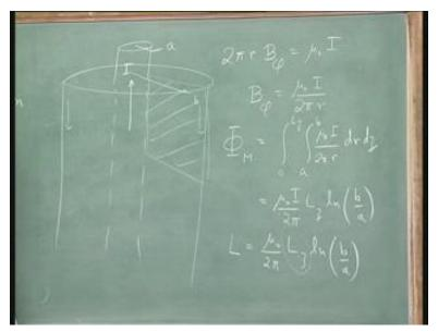
I have my inner radius of my wire is a outer radius is b. So the current goes let us say up i z in the inner wire and comes back down on the outer wire because there is a symmetry I can again calculate b. Stoke's theorem tells me 2 pi r b. Since the current is in the z direction b is in the phi direction is equal to nu naught i. There is only one turn. This is not a case with n turns, a single turn single wire is going up and coming back bringing everything back.
