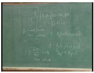
We looked at an irregular solenoid and we concluded that the magnetic field is constant inside and 0 outside. We did that by proving that the magnetic field is in the z direction and then if it is in the z direction, you can always draw Stoke's loops and since there is only magnetic field here and here you have loop integral b dot d l is equal to b of r 1 minus b of r 2 times d l. But, there is no current entering. It is supposed to be equal to surface integral j dot d s which is 0.
