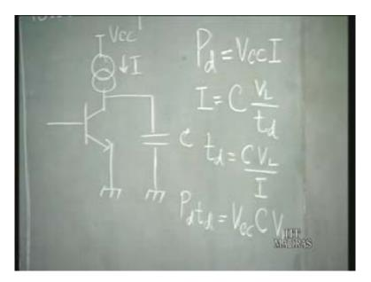
So what is the delay when this capacitance is charged with a current source of value i? When you are charging a capacitance i is equal to  $c_d v_d$ . So if you write i is equal to c, so the change in the voltage is  $v_L$  which is the logic swing and the delay will be given
