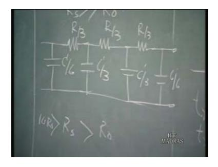
These are resistances of the line. Basically we do not have a single resistance and capacitance but this is distributed and we find that this gives the more accurate delay values for the line. In fact if we take the lumped value that is only one resistance and one capacitance then it is going to something like this is for lumped.
