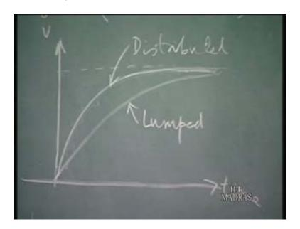
If you take a distributed value it goes like this. This is voltage versus time, so this is distributed. This gives the more accurate representation and the lumped representation gives a higher delays than what is to be expected normally.
