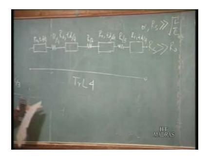
You have a four section transmission line model, this is called trl transmission line four model. Now if you have one transmission line section that will be the trl one model. When the resistance of the line is small, you can take the one section transmission line model but if the resistance of line becomes large, we have to go for the four section transmission line model which includes the effect of the resistance of the line that is basically considers lossy transmission line.
