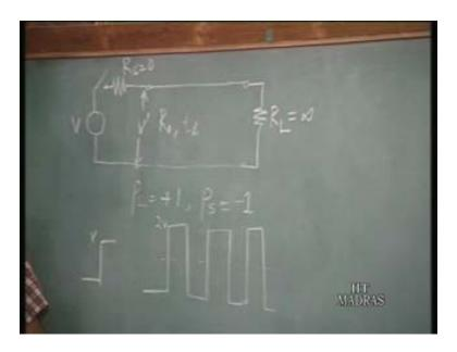
That is when we close this switch here, we get a waveform as step input at the source end of the line. The output is going to be something like this oscillations and which are not going to die down of amplitude twice V. This is of course going to be a very bad situation and of course this is the extreme case that is one end short circuit and the other end open circuit.
