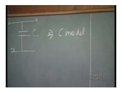
If you have just this model which is called the C model and if you consider open circuited line at the load end then we know that the output voltage  $V_{\cdot 0}$  is equal to V (1-e to the power minus t by  $R_{\cdot 0}$  that is the source resistance into C prime.
