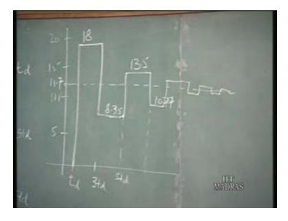
If this is 10 volts, 20 volts, 5, 15 volts so the waveform goes all the way up to 18 volts at  $t = t_d$ . Here again we come back to this diagram. This 0.8 volts has gone back to the source end. Now again this is going to get reflected from the source end with a
