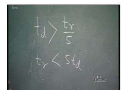
In other words we can also say when the rise time is less than 5 times the delay time of the line then one has to actually look into the transmission line effects. This is the rule of thumb which is used to demarket, when the transmission line effects are dominant or when we can neglect transmission line effects. Now if you look at the different rise times for example if you have a rise time of say in picoseconds say if you have 1000 picoseconds that is one nanosecond of rise time.
