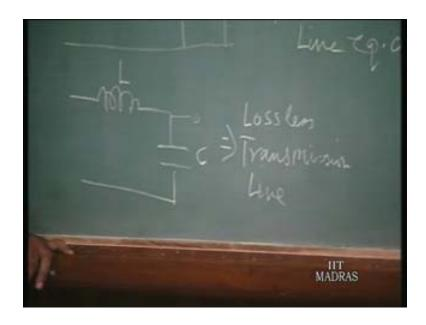
We shall first take up the effect of this lossless transmission line on the performance of integrated circuit and then we shall consider the effects of say for example the resistance on the line subsequently.
