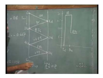
I will write it here is 0.8 and at the source end rhos is equal to - 0.667. The reflected wave here is 0.8 times the incident wave.
