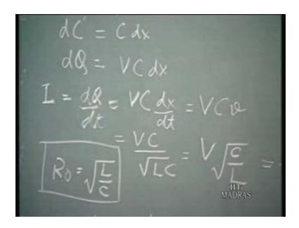
What is the extra charge that is required? That is this is the capacitance, the voltage which is charged by voltage V so V C dx that is the total charge and therefore the current is given by we know dQ dt so we get VC into dx dt which is nothing but the velocity.
