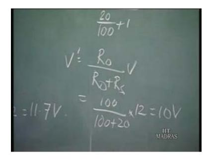
A voltage front of 10 volts is available here at the source end of the transmission line which is going to move towards the load end of the line. If we come back here in this diagram this is at time t=0 and at time  $t=t_{\rm d}$  you have a 10 volt. This 10 volt front moves and reaches the loads end. Now this gets reflected and the reflection coefficient is at the load end rho<sub>L</sub>.
