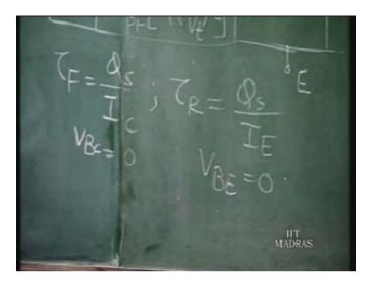
What is the transit time? The transit time as we had defined it is the ratio of the charge stored to the current. In this case, the forward transit time is given by so when we define all the forward parameters are defined for  $v_{BC}$  equal to zero. So when you define tou<sub>F</sub> which is the forward transit time it is for  $v_{BC}$  equal to zero, so you don't have the reverse the charges due to the base collector junction. So that is given by Q by the
