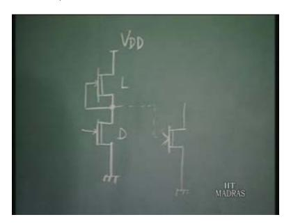
This is the driver transistor and this is the load transistor and for the load transistor, the gate to source is shorted and so  $V_{GS}$  is equal to zero and by adjusting the  $V_{DD}$  we can again ensure that the load transistor is always in the saturation region. Now this circuit has a certain problem. Suppose this has to drive another similar inverter.
