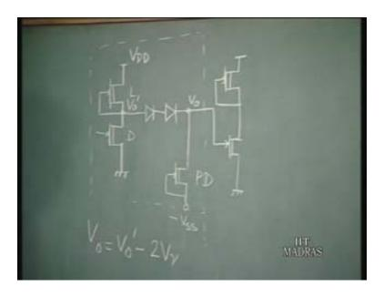
A current will always flow through this pull down device. What is going to happen because of this drop across the diodes, so this voltage here is going to be level shifted by two diode drops. If we call this output voltage V.o. prime say, this actual output voltage here is going to be V.o. and V.o. is always going to be V.o. prime minus twice we can call it v.gamma where v.gamma is actually the cut in voltage of the diodes. There is going to be a level shift between these two devices.
