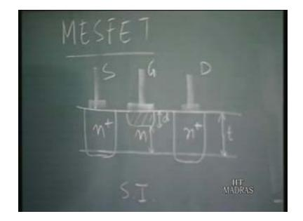
A schottky diode is a metal semiconductor junction diode and it behaves as a normal diode, the characteristics is like a normal diode and it has got a cut in voltage. If the voltage across the device, forward bias across the device exceeds the cut in voltage, there is going to be conduction. If the characteristics of the schottky diode is just like another diode, it is something like this.
