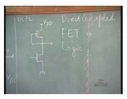
Now this circuit consist of an inverter, this is the basic inverter for this logic family. It consists of an enhancement type driver transistor and a depletion type load transistor where the gate to source of the load transistor is shorted. If you take such a circuit and consider that this is connected to the input of another gate that is basically one inverter driving another inverter, let us look at characteristics of this logic family.
