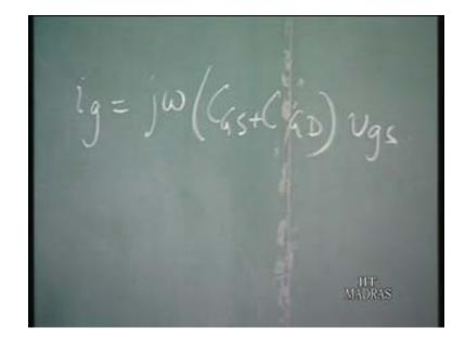
ID is equal to  $g_m v_{gs}$  therefore AI modulus of the current gain is equal to  $g_m$  by omega CGs plus CGD.
