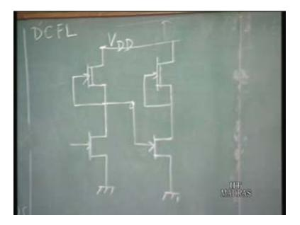
Let us go back and draw the load line again. Draw the characteristics and the load line to obtain the input output characteristics. We have the IV characteristics of the driver transistor and what we do is we draw the IV characteristics of the load which is a depletion mode load at  $v_{\rm gs}$  is equal to zero.
