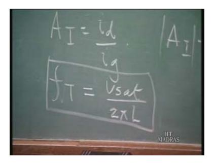
The frequency at which the current gain is going to go to unity is  $v_{sat}$  by twice pi L. This is the  $f_t$  of the device. Now usually the  $v_{sat}$  of the MESFET is around 10 to the power 7 centimeter per second. So if you have L of 1 micron which is 10 to power minus 4 centimeter.
