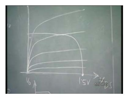
This is the characteristic of the load device. Now in this circuit let  $V_{DD}$  is 1.5 volt that is usual voltages at which the DCFL direct coupled fet logic circuits operate. Now another point to note here is that this output of this inverter is actually driving the input of the next gate. If we come back to the cross section view of the MESFET what we have is a schottky diode.
