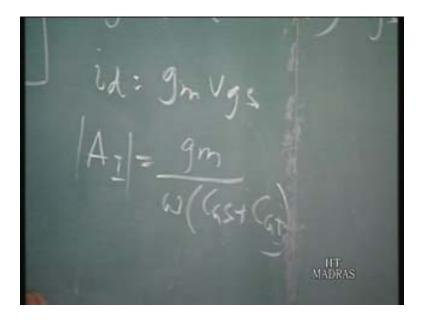
Now  $C_{GS}$  plus  $C_{GD}$  that is the total capacitance can be written as  $C_{GS}$  plus  $C_{GD}$  is equal to w into l that is the area epsilon by the depletion width.
