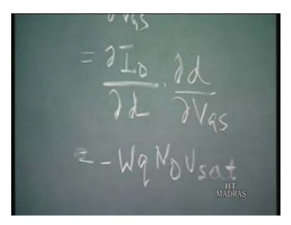
Now from this relation del I<sub>D</sub> by del d will be equal to minus w q N<sub>.D</sub>. V<sub>.sat</sub> and now we have to look at variation of d with respect to  $v_{gs}$ . If we assume that the depletion layer width is almost a constant from the source to the drain end, we can write that d is equal to twice epsilon that is the  $v_{.bi}$  is minus  $v_{.gs}$  by q N<sub>.D</sub>. This is the drop across the depletion region.
