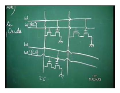
Again at every intersection you have a cell. This cell is basically a two transistor cell unlike the other ROM which are one transistor cells. It is something like this and of course at every intersection you have this. Now what is the purpose? Here you see one is the word line, you have two word lines in fact.
