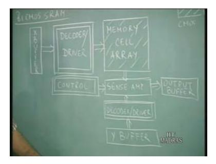
For example in the memory cell array because of the fact that the CMOS is a more dense circuit that is it requires less area, at the same time the power dissipation is less. We would retain the CMOS for the memory cell array, the decoder drivers are BiCMOS because the BiCMOS is capable of driving very large capacitive loads and we have a very large capacitive loads. The word lines and the data lines represent very large capacitive loads.
