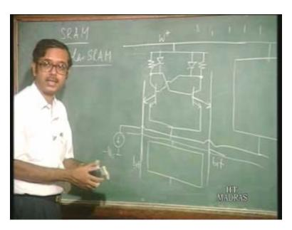
Similarly on this column you are going to have other cells or there are different word lines to energize these different cells in this particular column. This is one particular cell now let us see how this memory works. For a memory you basically have three states, you can say or 3 conditions. One is the holding state where you just retain whatever is stored in the memory, the same information is retained. Basically you are not reading or writing, you are just holding whatever is in the memory.
