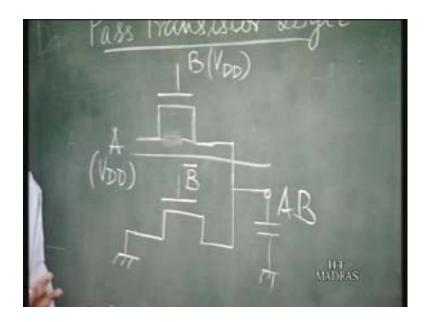
Now what you have? When B is high, output is A that means if A is also high, output is one. When both are high then only the output is one, if B is high A is 0, output is 0. When B is zero then this is off, this is on (Refer Slide Time: 25:46). So output is 0, so only when A and B are both high then only the output is high so it is a AND gate. You have realized an AND gate with the pass transistors.
