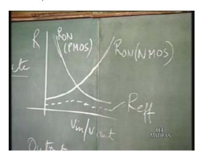
The PMOS was off because the gate to source voltage was zero but as this voltage is rising, the gate to source voltage is becoming more and more negative. Gate is zero, the source is becoming more and more positive, so the gate to source voltage is becoming more and more negative. So for the PMOS since the gate to source voltage is becoming more and more negative, the resistance is falling. We will plot for the PMOS, you have something like this Ron for the PMOS.
