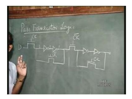
D flip flop is just a D flip flop with which is enabled when the clock is high will pass the input to the output when the clock is high and when the clock is low, the previous output is going to be retained. That is very easily realized using a pass transistor. This is the D input and say this is the clock here and you have two inverters and here you put clock bar.
