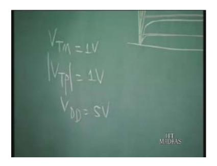
So let us write like this, modulus of  $V_{.Tp.}$  1 volt also and  $V_{.DD.}$  is equal to 5 volts. Let us take this particular case and these characteristics, so 1 volt is the threshold voltage. So let this be for say 1.5 volt say 2 volts, 2.5, 3, 3.5 and so on. This is for the NMOS transistor. So these are the characteristics for the NMOS transistor, gate voltage of 1.5, 2, 2.5, 3, 3.5.
