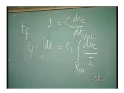
Now this is  $C_L$  so initially what happens is the input is high. So this NMOS input is high, output is also high. So  $V_D$  the drain voltage  $V_{Ds}$  might be greater than  $V_{Gs}$  minus  $V_{T.}$ . So it means that this transistor is in the saturation region. So this transistor is initially in saturation and then as the capacitance is discharging, the output is falling then it comes to the linear region.
