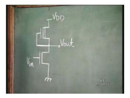
So the structure of this is something like this. This is a depletion mode MOSFET, the symbol is something like this. We put an additional line here which signifies it is a depletion mode MOSFET and for this MOSFET, the gate and the source is shorted for the load transistor. So here it is v<sub>in</sub> and here you have v<sub>out</sub>. So this gate and source is shorted. Now we shall again try to do what we have been doing graphically that is
