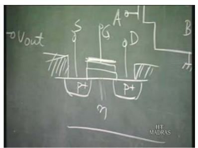
First what is a pMOS? The pMOS is again a MOSFET where the source and drain regions are made of p plus material. The substrate is n type, so this is also an enhancement mode device. So it is exactly like an nMOS, only thing is that the p regions are replaced with the n regions and the n regions with p regions and since the charges, the nature of charges, the sign of the charges are being changed, the voltages required to operate this device are just the opposite. That is the wherever you have
