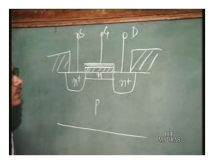
So that between the source and drain there is going to be conduction when drain voltage is applied even when the gate voltage is zero. This is a normally on transistor, the other transistor where the channel does not exist is called an enhancement mode device where it is a normally off device, when the gate voltage is zero the current is zero. This type of transistor is also called a buried channel MOSFET because of the existing already existing channel bc MOSFET sometimes.
