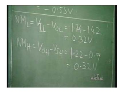
So that is minus 1.22 and the logic high output is 0.9 volts minus 0.9 volts. So the noise margins are symmetric in this case for 0.32 volts. So we have made the calculations of noise margin from here. Then the next thing which we shall take up from the circuit is power dissipation.
