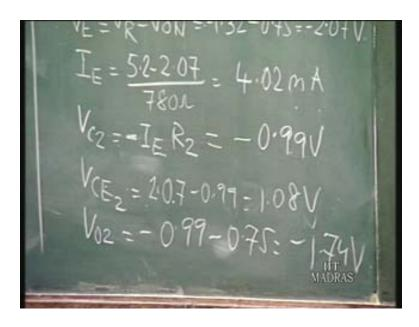
So what is V output?  $V_{.02}$  minus 0.99 minus 0.75 is equal to minus 1.74 volts. So that is the output when in this condition. That is  $T_2$  is on and  $T_1$  and  $T_3$  off and what is the output at
