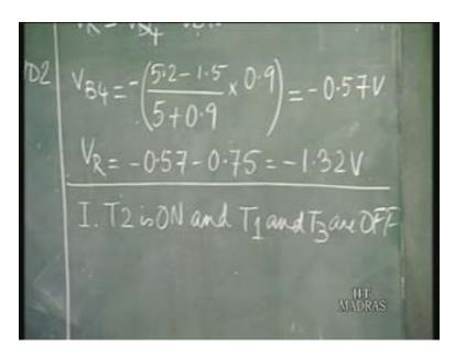
Now we shall look at the two different states that is one is when the left branch is conducting and the other is when the right hand branch is conducting and the other is when the right hand branch is conducting. So let us say case one, T<sub>2</sub> is on and T<sub>3</sub> and T<sub>3</sub> are off that is the right
