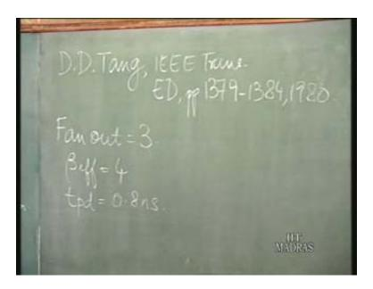
The results which they gave, came out was for a fan out of 3, for this particular structure for fan out equal to 3 that is for 3 collectors. They had a beta effective equal to 4 and interestingly the propagation delay of 0.8 nanoseconds. At collector current of I<sub>0</sub> equal to 100 microampere.
