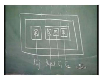
So you have an injector here, this is the injector, this is the input or the base it's also sometimes called the base contact, it's the collector C one, C two, this is the two collectors here (Refer Slide Time: 15:25). So this is the mask drawing or the top view and this is the
