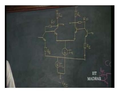
Therefore you have the differential integrated circuit version of the so called voltage controlled voltage source. The only thing is, if you want the gain as  $R_F$  by  $R_E$  you have to
