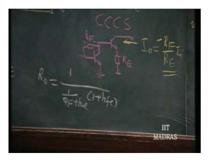
Similarly, for the differential structure the output impedance depends upon  $R_F$  and the hfe of the transistor. Now we know the input impedance, we know the output impedance and we know the voltage gain. Therefore we know all the small signal parameters of this wide band amplifier. You must also analyze the voltage swing etc because this wide band amplifier may be ultimately amplifying large signals. So I would like you to evaluate the DC voltage at this particular point. It is very easy.
