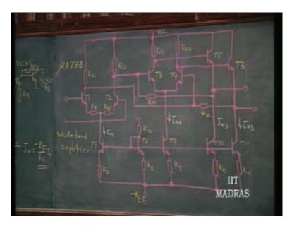
Next we have the second stage which is nothing but this structure. Here we have  $I_{01}$  which is....and finally  $I_{03}$  is through the common collector stages and in the final output stages we have  $I_{03}$ . Try to do the analysis of the circuit not neglecting anything but considering all the non idealities into account that means beta is not infinity or alpha is not equal to 1 and then consider all the effects of other transistors in evaluating the gain or the loop gain etc.
