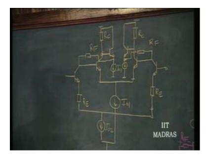
Let us identify the current sources and the respective transistors. The transistors are  $T_1$  and  $T_2$  and the current source that is  $I_{02}$  is this. That is obtained by a reference that is getting generated. This is a transistor connected as a diode so  $V_{EE}$  minus V gamma by  $R_{12}$  plus  $R_8$  and you can accordingly fix the voltage here so that you obtain the desired current by adjusting  $R_7$ . So this is  $I_{02}$ .
