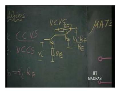
Again it is a wide band structure. And this is what is utilized in one of the most popular wide band structures called [] this wide band amplifier which is called muA733. If I have to convert this into a differential configuration path bias purpose what should I do? If I have to convert this into IC so that biasing is taken care of automatically without the need for bypass capacitors and coupling capacitors then what should I do to this?
