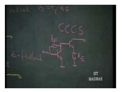
Therefore the current gain is, if this is the input current Ii this current will go into this  $I_i$  into  $R_F$  and that will be divided by this which means current will be going into this stage and it is going to be  $I_0$  is equal to  $R_F$  by  $R_E$  into  $I_i$ .
