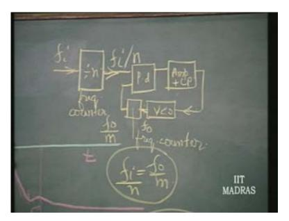
So what happens here is, phi by n is equal to  $f_0$  by m these two frequencies should become one and the same. So  $f_0$  is equal to mfi by n. So by using this combination of two programmable counters I can manage to get any m by n, m and n are integral values.
