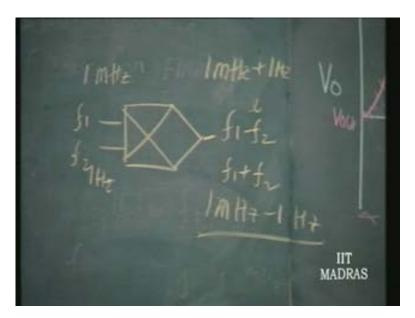
Therefore what you must do is, put this in a Phase Locked Loop that is what is called frequency translation effect. You have to use a multiplier but multiplier must be part of the loop. Let us see how it is done.
