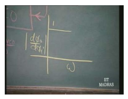
If there is no change in phase there is no frequency but if there is change in phase there is frequency. Now this frequency itself can change that means there will be FM. That means, if I give an FM here and that FM is modulated at a certain frequency it is that
