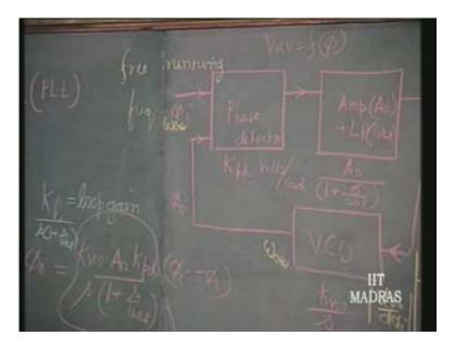
Suppose I give  $omega_0 Q$  here this is  $omega_0 Q$ , this is  $omega_0 Q$  now what should happen is, according to the principle of Phase Locked Loop there is a same frequency and nothing should happen, that is this frequency should not change because I am feeding the same frequency at the input which means the output here should be zero. That means the control loop should adjust its output so that this is zero, when does it happen?
