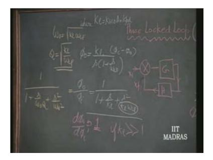
Now this is important,  $K_1$  is what is called as the DC loop gain, root  $K_1$  into omega<sub>LP</sub> is called the natural frequency of the phase locked loop and if you plot this magnitude of phi<sub>0</sub> by d<sub>i</sub> versus the frequency of change of phase, the phase is the input here but that phase itself can change at a certain frequency that means it is called, phase is changing at a certain rate that is called frequency and that itself can change that means it can be a FM.
