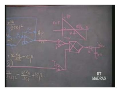
This was the phase characteristic with respect to, this is pi by 20. So we can find out whether it is tuned to the incoming frequency or not the moment we get a zero average voltage at this point. Now how do I therefore make sure that this is going to be the case automatically?
