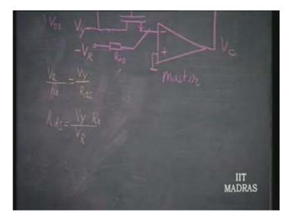
It is necessary that  $V_Y$  can only take on the positive polarity in this case if this is my negative. If this is positive this has to be negative, this is the requirement. Under this situation  $V_R$  by  $R_0$  is equal to  $V_Y$  by  $R_{ds}$  or this can be written as  $R_{ds}$  you replace  $R_{ds}$  is equal to  $V_Y V_R$  by  $R_0$ . If you now replace this  $R_f$  by  $R_{ds}$  which is  $V_Y$  into  $V_R$  by  $R_0$  into  $V_X$  this becomes a div<sub>i</sub>der in this case.
