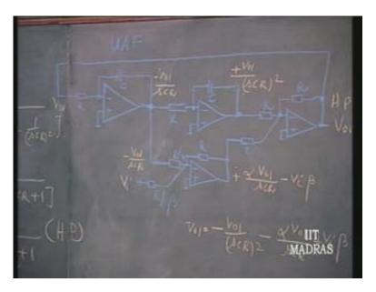
If you take the output here this is then the high pass and that high pass output into 1 by sCR or  $omega_0$  by s minus which will give you band pass. So  $V_{02}$  by  $V_i$  is nothing but minus s by  $omega_0$  beta divided by the same denominator which is band pass.
