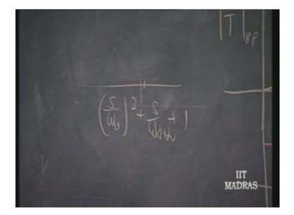
You can just put this as s is equal to j omega and omega is equal to omega R. Therefore, as far as the numerator is concerned we are not bothered but as the denominator is concerned we know that as omega R is very low what is the phase shift?
