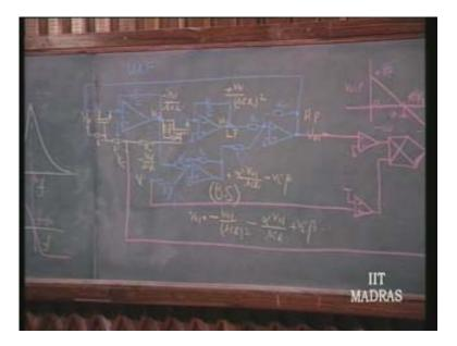
This is an automatic frequency locking scheme, it is automatically self tuned. This voltage has to automatically become equal to 0. If this is a negative feedback system since I am using an op amp here this output should adjust itself so that this voltage and this voltage become one and the same if it is a negative feedback system which you have to make sure. The proper polarity has to be put here to see that it is a negative feedback system.
