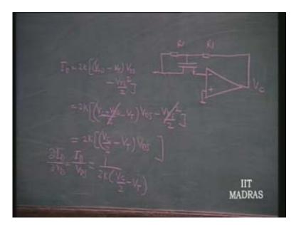
So in any case this demonstrates a particular method of making the FET linear, the  $V_{DS}$ .
