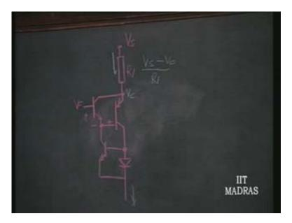
So now I have a current mirror coming to my rescue so I will put a current mirror here so as to make this operate at the same current as this. Therefore this transistor and this transistor are operating at the same current and if I now connect this the current leaving this is going to be  $V_s$  minus  $V_c/R$  and this is going to be same current, and here it is  $V_c$
