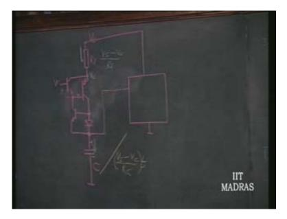
I want to charge a capacitor now so let us say I will connect this current over to the capacitor so what happens now is this capacitor is going to get charged and the voltage is going to increase at a rate which is nothing but  $V_s$  minus  $V_c/R_c$  into t. This voltage is now going to be buffered that means you can use a common collector stage and connect it over to.....
