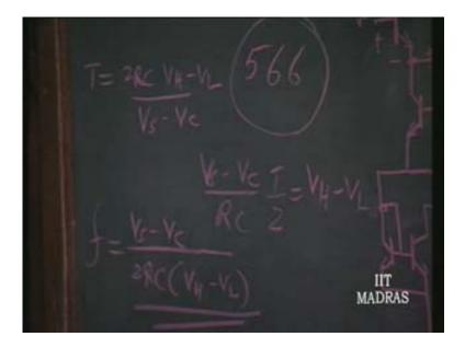
The other VcO is what is called Emitter Coupled Multi-vibrator which is also a multivibrator kind of a thing used in some other PLLs. Emitters are coupled by means of a single capacitor and there is regenerative positive feedback from collector to base and collector to base.
