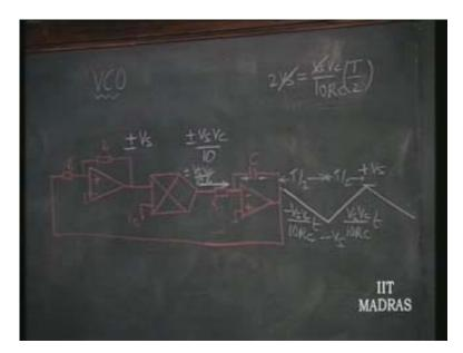
Now this is the frequency of oscillation of our  $V_c$  over here which is going to have a triangular waveform here and square waveform here. Now the important parameter associated with the VcO is delta f/delta  $V_c$  or this is called  $K_{VcO}$  or it is called VcO sensitivity.
