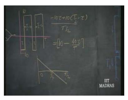
What will it be on this side for the negative? The same thing so it repeats itself. This is the characteristic of this phase detector because it is not able to distinguish between phase lead and phase lag, so because it is not able to detect this kind of phase lead or phase lag we are necessarily required to locate our quiescent phase shift at  $\pi/2$ . That means we subject one of the inputs to an additional phase shift of  $\pi/2$ .
