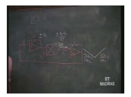
Only when this voltage becomes same as this voltage it gets into the regenerative feedback mode it goes into the active region where it has the regenerative feedback and therefore immediately it will change state from plus to minus. So what happens is, this is going to be plus  $V_s$  and this is going to be minus  $V_s$ .
