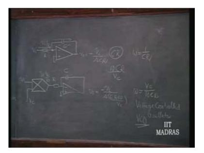
Therefore that is a double integrator oscillator and if you replace it by this the frequency of oscillation of the double integrator oscillator is going to be omega is equal to 1 by CR whereas in this case it will be omega is equal to  $V_c$  by 10CR. That means it becomes a voltage controlled oscillator. It becomes a linear voltage controlled oscillator or VCO. The frequency of oscillation can be linearly controlled by varying  $V_c$ .
