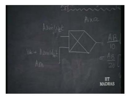
So, by nearly changing the input I am getting different applications. For AM generation the input will be this and for balanced modulation the input will be this. If on the other hand,  $\text{omega}_1$  is  $\text{omega}_C$  plus or minus  $\text{omega}_m$  and  $\text{omega}_2$  is  $\text{omega}_c$  plus  $\text{omega}_{IF}$  what happens?
