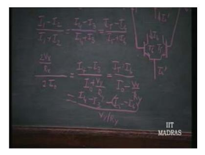
So we get  $I_4$  minus  $I_3$  minus  $I_5$  minus  $I_6$  by  $V_Y$  by  $R_y$ . that means this relationship is same as this whole thing which is  $2V_X$  by  $R_X$  by  $2I_0$  equal to that is the final relationship  $I_4$ minus  $I_3$  minus  $I_5$  plus  $I_6$  if you remove the bracket so ( $I_4$  plus  $I_6$  minus bracket  $I_3$  plus  $I_5$ ) rewriting the same numerator we get this as ( $2V_y$  by  $R_y$ ).
