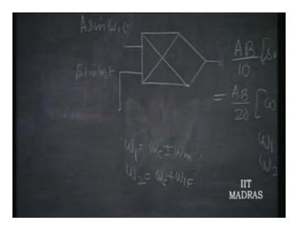
In the difference component you will get  $\text{omega}_c$  going and it will be  $\text{omega}_{IF}$  plus or minus  $\text{omega}_m$ . There will be of course two  $\text{omega}_c$  components plus  $\text{omega}_{IF}$  plus or minus  $\text{omega}_m$  component the other one. That can be got rid of by using a band pass filter which is called IF filter, this is called IF filter. That means at that point of time this is
