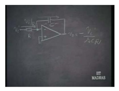
Voltage controlled amplifiers can in turn be used, this is an op amp integrator when this is  $V_i$  the current in this is  $V_i$  by R it will flow through this and develop a voltage which is  $V_0$  is equal to minus  $V_i$  by SCR so it is an integrator. An integrator is one of the most important basic building blocks in analog signal processing particularly in what is called filtering. Therefore an integrator is an important building block.
