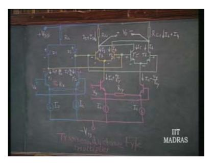
And therefore if this current being  $I_0$  and this current being  $I_0$  this will be  $I_0$  plus  $V_X$  by  $R_X$  and this will be  $I_0$  minus  $V_X$  by  $R_X$  where a differential current is generated. So if you replace this  $I_1$  and  $I_2$  by these two currents now we can see here that  $I_1$  minus  $I_2$  is nothing but, let us say this is our  $I_1$  and this is our  $I_2$ .
