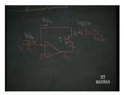
So purposely we put the emitter degeneration resistance. So we will increase the emitter resistance by putting additional resistance here so that the gain now is  $R_X$  by  $R_E$  plus  $R_{E1}$ . You can reduce the gain to almost nearly 1 and therefore resurrect this amplifier which was going to oscillate otherwise because of its inherent frequency compensation being valid for its maximum loop gain of A.
