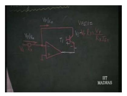
What we are now designing is nothing but a log amplifier. Given the input voltage  $V_X$  it is going to give an output here which is nothing but minus  $V_t \log V_X$  by  $R_X I_{E0}$  whether you put a resistance or not. You do not put a resistance; nothing is going to happen because current is going to be limited to  $V_X$  by  $R_X$ .
