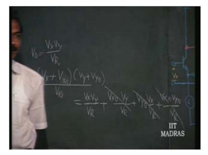
Now this is behaving like a non ideal output in the case of a multiplier. So what should you do is you should subtract DC. Subtracting that DC is not a problem, it is only a DC and you already have  $V_Y$  and  $V_X$  with you. So some portion of  $V_X$  and some portion of  $V_Y$  have to be subtracted from this. Using op amp I want you to obtain a generalized single quadrant to four quadrant block.
