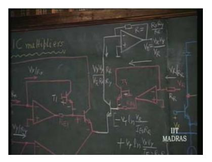
Now you see how neatly this is working. This current can be made to go through another resistor of an op amp which is connected in a similar fashion. This current will therefore be converted to a voltage, so what will be the output voltage now?
