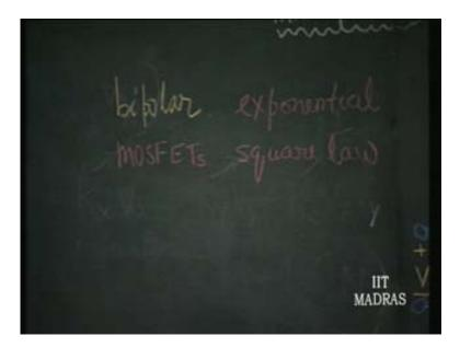
What are the basic methods of multiplication? Now we will consider the devices that are available to you. The nonlinear devices that are available to us are bipolar transistor and MOSFETS. Bipolar is essentially a nonlinear device which is using exponential relationship. The I is equal to IA<sub>0</sub> exponent  $Q_v$  by K<sub>t</sub> minus 1.
