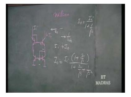
That means this kind of concept can be therefore straight away used in PNP configurations where beta value is known to be lower. Now let us see the other negative feedback concept that we can utilize.
