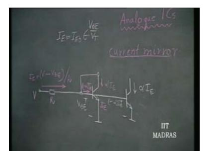
The idea is very simple. As the name itself indicates mirror is something that reflects the image exactly in an identical fashion, Replica of the original stuff of whatever it is. In this case it is a current mirror. It should exactly reproduce the current that is existing originally. So what is it, how is it made?
