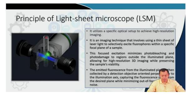
So, basically this is what is happening the this is the sample box where you have your particular sample and it is illuminated from this side it is illuminated from this side it is illuminated from this side and at a 90 degree you are doing the detection.
