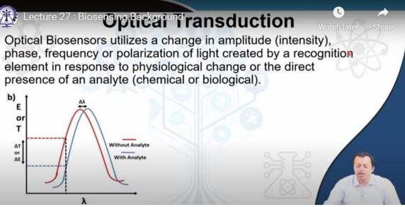
So, this is something that you detect the ah how much this lambda will shift with respect to change in refractive index previously the refractive index was 1 now you have put an analyte with a refractive index say 1.4 1.5. So, it is 1.4 minus 1 that is 0.
