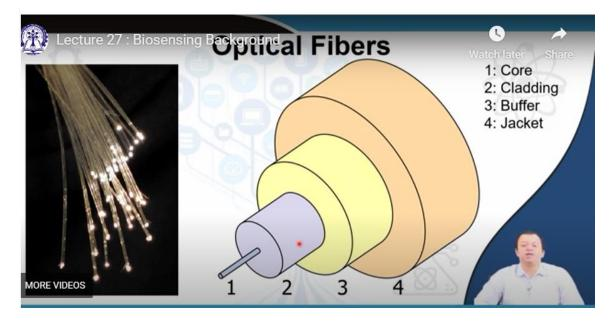
So, the first thing that they did was trying to work on optical fibers optical fibers as you know you have a core versus cladding higher refractive index lower refractive index and thereby you have total internal reflection optical fiber I do not want to go too much detail on to this, but for non medical people optical fiber is something that gives you the
