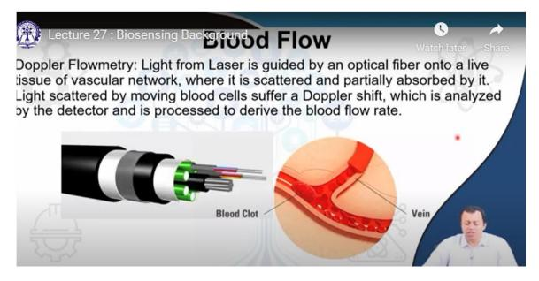
flowmetry has been used this is another fascinating thing light is being sent through several of these ah small cores into a vein into your vein you insert this light is being send and some of the light is being reflected and since there is a flow. So, this is a vein having blood flow and there is a blood clot you know about Doppler shift when things move away from it from you you have a red shift into the frequency. So, think
