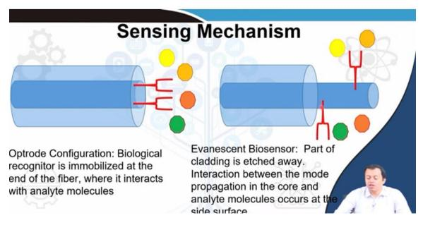
light is determined by the presence or absence of a specific antigen connecting with a specific antibody you can either put it at the top of the tip of the core or at the body of the core. Similarly, you can have you know structure such as this functionalized ah MNF
