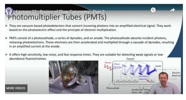
So, these are the PMT tubes the photo multiplier tubes they are vacuum based photo detectors that convert incoming photons into amplified electrical signals.
