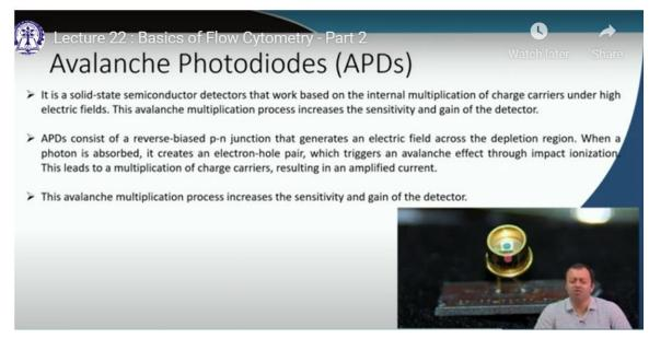
We can also do photo diodes these are something that I am more comfortable with avalanche photo diode it is a solid state device it is simply a photo detector light falls electron hole pair is generated electron hole pair are generated is separated away.
