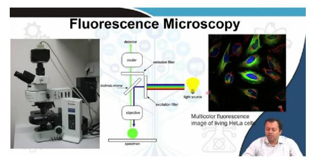
So, fluorescence microscopy is therefore, have been revolutionizing you have a light source that is filtered out a particular blue light is made to fall on a particular specimen that specimen contains fluorophore either directly connected with the biological material or it is connected via something blue light is the input the electron goes up goes through some sort of a transition returns back to the original place by emitting green light.
