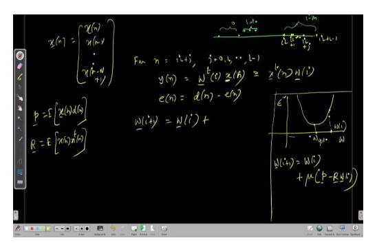
So, I should ideally follow this, but as I told you we will be replacing small p because p is not known to us we have to approximate it by some data value data driven approximation I have to do for p and R in the case of LMS we need a very bad approximation that time p
