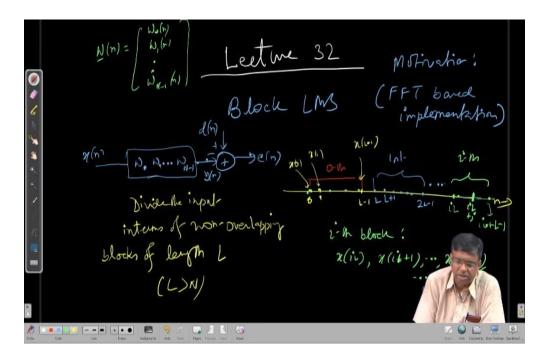
So, filter coefficients are updated only once per block and then held fixed within the block for doing the filtering operation ok. So, we will have Wi this is the filter weight vector for the Ith block and we will update update means Wi to next block. So, once I have Wi I will be using it at all the points within the Ith block all right. That means I draw that line again
