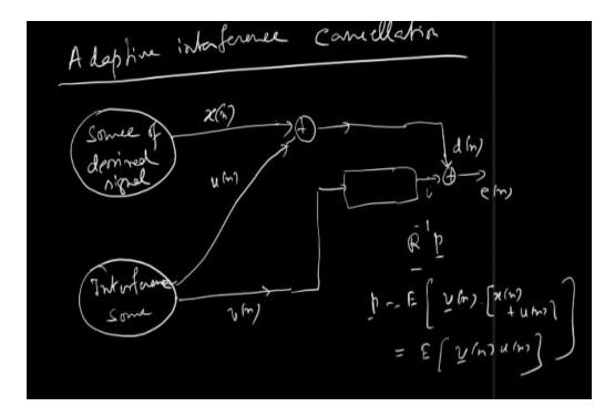
So, you will have a u cap n here ok. So, what will come out x n plus u n minus u cap n. So, u n and u cap n they are very close to each other. So, the residual interference which is u n minus u cap n will be very small close to 0 and what will I will what we will have here largely is x n.
