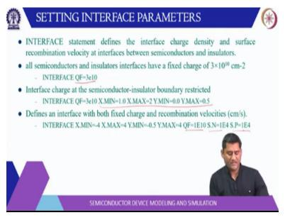
Interface statement it defines the interface charge density the surface recombination velocity how the recombination takes place at the surface. So, for example interface fixed charge is 3 into 10 so 10 per square centimetre. So, this many electrons per square centimetres are there electronic charge. The interface charge at the semiconductor insulator boundary. So, you can specify the
