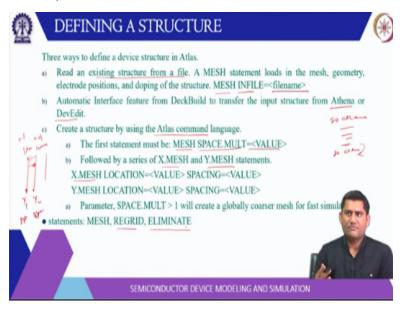
So, defining the structure, there are three ways to define a structure. One it can read an existing structure file. So, that structure file can be generated from the Dev Edit or you may have previously generated that file. So, you can read that structure file and the syntax is MESH INFILE and write the file name. File name usually as a extension.str. Another one is automatic interfacing with the Athena simulation.
