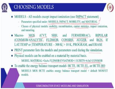
Then choosing the models. Models are chosen so all the models are especially around the model statement except the impact ionization. So, this impact ionization and models are specified using the impact statement. So, for example mobility material parameter they specify the parameters for these models. So, mobility and material parameters they are specified under the separated statement.
