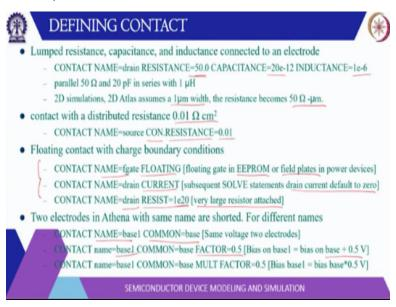
Now lumped elements can also be specified along with the contact name so, you can especially that like RESISTANCE 50 ohm CAPCITANCE 20 into e is 12 so that is 20 picofarad inductance 1e - 6 and 3. So, it is micro Henry. So, in 2D simulation your Atlas assumes one micro meter bits in the third dimension. So, the resistance will become 50 ohm micrometre you can also specify the distributed resistance.
