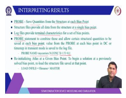
Then there is a probe command which allows the quantities to be probed at that particular position. So, from save quantities from the structure at each bias point you can have these quantities. So, structure file provides all the data at a single bias point. So, this is the effect of probe statement and log files provide the terminal characteristic for a set of bias points. And probe statements combine these two and allow certain structural quantity to be saved at each bias point.
