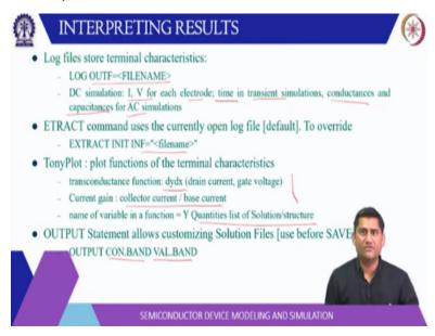
Then interpreting the results, the log file you can write the log out file name then in the DC simulation you will get the I, V characters for each electrode in transient simulation time is added and in AC simulation you also get the conductance and capacitance for each terminal. Then extract command you can extract the parameters from the log file or the structure file. Then Tony Plot basically it plots the IV characteristic.
