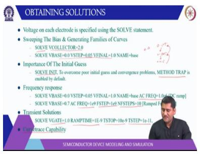
Then obtain their solutions you can write the command solve statement mention the internal name and especially the voltage or if it is a current contact then especially the current. The contacts that are not specified any value by default they are zero. So, you can solve VBASE and VSTEP it from 0 to 1 and the VSTEP size of 0.05 so, solvent is another command to create an initial guess. So, it basically to overcome poor initial cases and converges problem METHOD TRAP is enabled by default.
