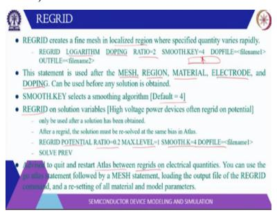
REGRID creates a fine mesh in a localized region where the specified quantities varies rapidly. So, for example you have a PN junction so at the interface the carrier consultation varies with a grid slope. So, then you would like to have a final mesh there and by chance you have not defined that mesh you can REGRID it basically. And then you can write logarithmic scale with doping ratio two. So, this is basically used to REGRID the mesh.
