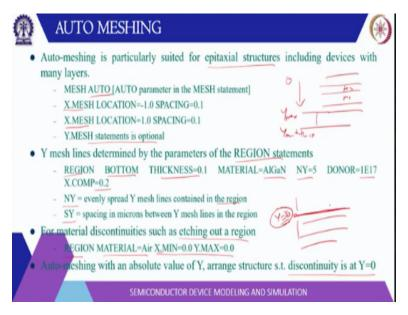
You can also use automation which is particularly useful for epitaxial structures because epitaxial structure you have to get you have to consider these different interfaces. So, this will automatically consider these interfaces from material 1 to material 2 and so on. Usually, the multi-layer structures like distributed drag reflectors big cells and so on. So, you can use the command mesh auto so auto parameter is there in the message statement.
