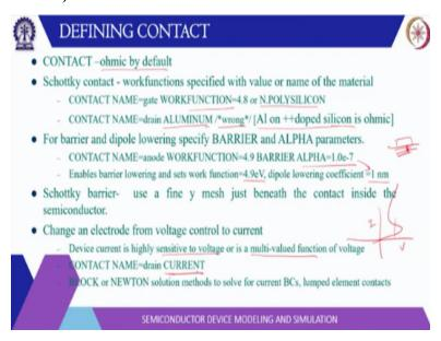
So, regarding the CONTACT it is ohmic by default. So, if you write a contact name then it will be assume to be ohmic but if we specify the work function or the name of the material. So, which has some associated electron affinity then that contact will deteriorate Schottky contact. But in case of aluminium to a highly doped region the contact will be ohmic only it will not be Schottky.
