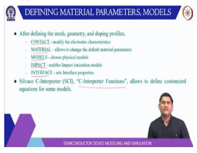
Then we are defining the material parameters and the models. So, there are statements here CONTACT, MATERIAL, MODELS, IMPACT and INTERFACE. So, most of the models are specified using the model command and only the impact ionization based models are enabled using impact statement. Then you can also have your own C file to define a customized equation for some model that Silvaco also allows.
