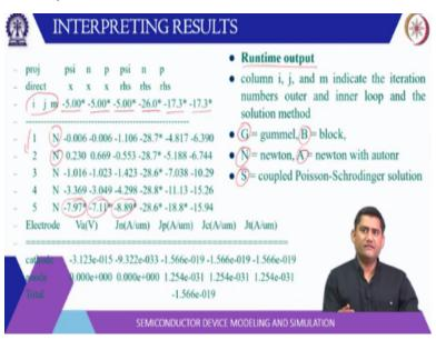
Now if you look at the typical output file you have this thing running runtime output you have these different i, j, m so, these are basically different iterations 1, 2, 3, 4 this method is Newton here so, it can be gummel block or Newton or Newton with autonr or couple Schrodinger Poisson. So, these may appear here and this i j m will represent the number of loops and these are the parameters for the convergence.
