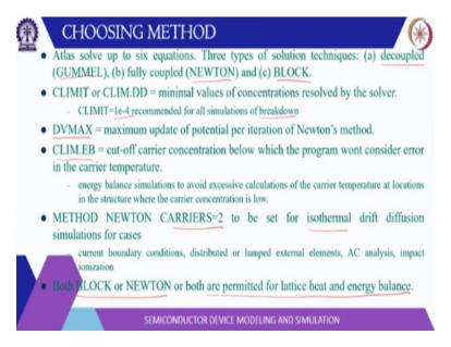
Then choosing the method, you can there are three methods that are available. If the equations are decoupled then you can go with the GUMMEL model and for coupled you can use NEWTON or the BLOCK method. For all the equations that are coupled then you can use Newton method and it is also default. Then the parameters also can be changed for example if you are doing simple PN junction simulation or device simulation you are okay to ignore some carrier consultation which is below certain limit.
