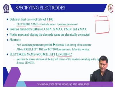
Then specifying the electrode, so again at least one electrode has to be specified and it will also be integer one and so 1, 2, 3 like that up to 100 you can specify. So, electrode name then mention the name and then the position parameters. So, position parameters again you can specify X MIN, X MAX, Y MIN, Y MAX so this is your structure. So, you can specify so this is X MIN this is Y MIN and Y MAX and so on.
