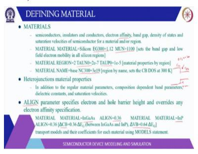
Then defining the materials, semiconductor insulator conductors they can be defined and you can change their properties such as electron affinity, band gap, density of a state for conduction band balance band saturation velocities mobilities. So, all these parameters can be modified under the material statement. So, you write the material then the name and the band gap and then this MUN which is basically electron mobility, this is a band gap 300 at 300 Kelvin.
