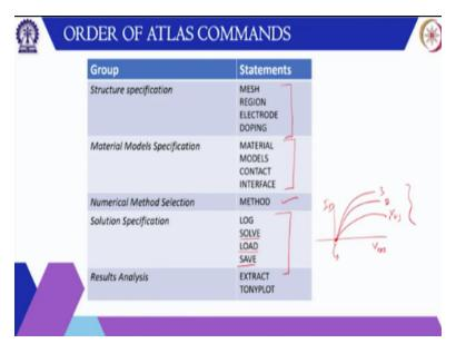
Now these are different groups we will go from through them one by one. So, you especially the mass the reason the electrode the doping then especially the material parameters. So, material their models the contact properties interface properties then select the numerical method then for solution you can specify the log file name then different solve statement. You can also use this load function this is basically used to set the initial solution.
