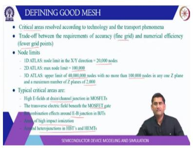
Then defining a good mesh. So, these are the summary of defining good mesh critical areas should be resolved according to the technology and the transport phenomena then trade-off between the accuracy and the efficiency. So, fine grid means it will have greater accuracy and
