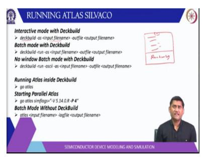
So, there are two ways basically, one of course you can open the deck build directly and write your code and there is a run button on it you run and it will run basically. Then you will have runtime log here and then if you specify any log file such as the structure file log file, they will be the output of this code. Another way you can run this drag build in interactive mode by using a command.
