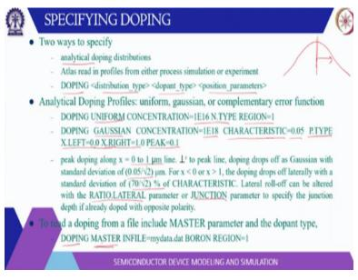
Then to specify doping there are two ways you can do you can specify the analytical doping distribution or it can read some input file so if doping profile is stored in file. So, it can read that profile from that file which might have been obtained through some process simulation or from
