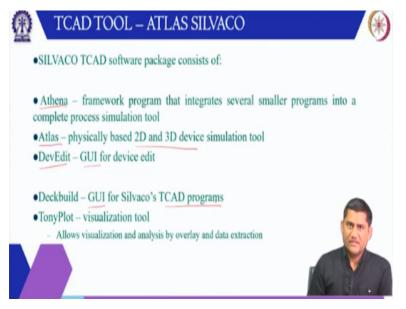
Now let me introduce the SILVACO ATLAS TCAD tool. So, this SILVACO TCAD software is consists of a process simulator which is Athena. So, it is a framework program so which integrates several small programs. So, there is a program for oxidation simulation, there is a
