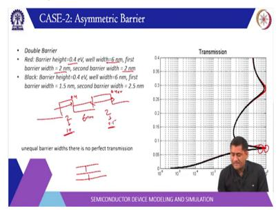
Now, let us consider the asymmetric barrier, so, here there are two cases, basically. In the first case, barrier height is 0.4 well width is 6 and the first barrier width is 2 nanometre second barrier with this also 2 nanometre. So, this is the situation like this, you have barrier height is same. So, this is 2, this is 2 and this is 6 nanometre and height is 0.4. Now, what is done here?
