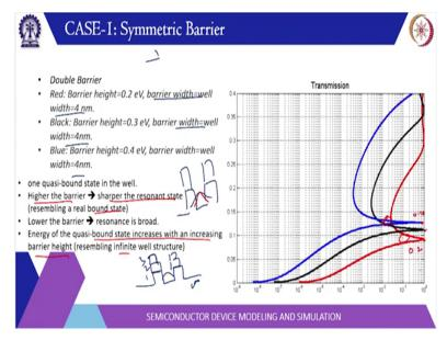
Then in a certain barrier we can also study, the effect of change in the barrier height, so, the barrier width and the well width are same. So, both are 4 nanometre here but the height is changing. So now, this scenario is basically like this. You have let me put it here, so, this is the first case, this is the second case and this is the third case. So, this is what happening here 1, 2, 3.
