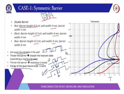
So, here you can see the case that case of that I have studied using this transform matrix approach. So, there are symmetric barriers, so, there are two various of same height, 0.3 electron volt, 0.3 electron volt and the well width is also same 4 nanometre, 4 nanometre only thing that is changing the height of these barriers. So, in first case the height is 2 nanometre in second case the height is let me use different colour second case height is 4 nanometre.
