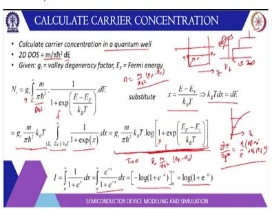
So, let us calculate the carrier concentration in a quantum well. So, as you know that quantum well is a kind of it is constrained in 1 dimension. Let us say this is the z dimension and in x and y direction it is free. So, there will be the z direction that means the k z will be quantized and k x and k y can take any arbitrary value. Now, if you recall, we calculate the density of a state for 2D system and it was m by pi h bar square.
