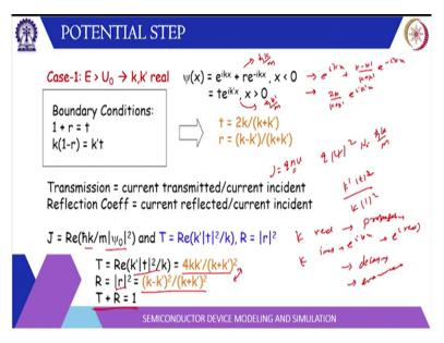
So, it is shown here the t is 2k by k + k prime and r = k - k prime by k + k prime. So, using you can write that your psi is basically e to the power iota kx + k - k prime by k + k prime e to the power –iota kx. And this is 2k by k + k prime e to the power iota k prime k. So, these are the wave functions basically. Now, the current is calculated in terms of the wave function. Wave function psi square tells you the density of carriers.
