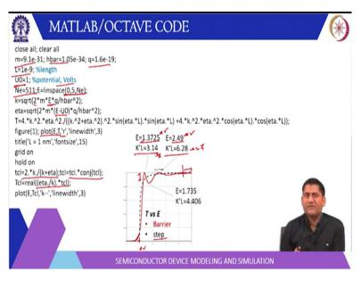
Now, you can write a simple Matlab code that I have done here. So, this is the mass of electron then h bar q the length is taken as let us say, 1 nanometre U naught is 1 unit is electron volt. So, what you will write here? We will multiply it by q so that is electron volt then number of steps 0 to 5 volt potential is taken, energy is taken and there are 511 elements are taken. Then case root 2mE by h bar square, so, energy is assuming electron volts.
