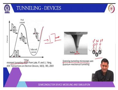
So, some devices that use this phenomena one is of course the resonant tunneling diodes. Other is the scanning tunneling microscope. So, there is a tip here which has also atoms here at the surface, there are atoms here. And they can measure the atomic distance because it is very sensitive to the barrier. So, this is basically barrier, so, there is a atom here and these are surface atoms, so, you see, this is a distance here, this is distance here.
