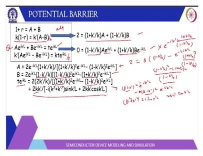
These are the four boundary conditions. We got two equations 1 + r = A + B k times 1 - r = k prime A - B. And if you divide second equation by k and add so on left side, you will get two on right side A times 1 + k prime by k and + B times 1 - k prime by k. So, this is one equation containing A and B. So, we have eliminated r here, in second equation also, you can eliminate t.
