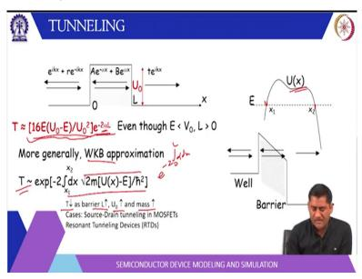
So, this understanding of the electron going through a potential barrier and the tunneling phenomena gives right to some kind of devices that they use the tunneling phenomena. So, since we have discussed this thing for a constant profile. Now, this principle can be applied to a general profile where potential is not constant, whether there is some function of position.
