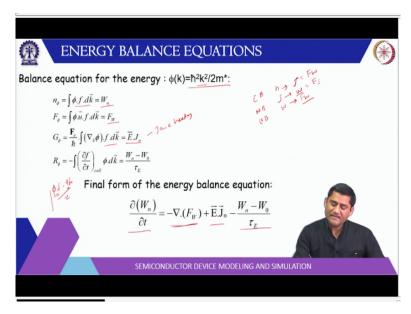
Now similarly we can draw the balance equation for energy by substituting phi equal to h bar k square by 2m. So, now n phi becomes h bar k square by 2m times f dk. So, that gives the energy density and the flux of the energy density is phi times u. So, it becomes k q basically and then generation is derivative. So, it becomes only instead of k square it becomes k. So, k f dk becomes J. So, f E times J is basically electric field times J and that you can say this kind of joule heating.
