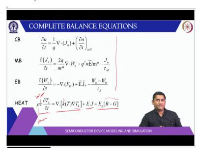
So, heat flux we can use phenomenological model. So, where you can say that the lattice temperature gradient del T L by del t is basically the heat flux plus joule heating plus the energy absorbed due to the recombination process. So, in the recombination this electron will combine and give energy equal to the band gap energy. So, E g times R and of course there is generation then this energy is taken away. So, we have R - G. So, this is electron voltage generation recombination.
