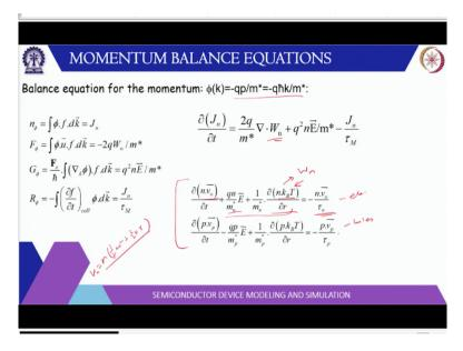
Now so if you substitute this phi, here we are substituting only qh bar k by m. So, if you take out the charge term here, if you just integrate with respect to h bar k you get d by dt of n v t + qn by E + n k T. So, this is the energy term. So, del I del r. So, the energy density is n k T because for single electron is half m v square + 3 by 2 k T and for n electron is multiplied by n.
