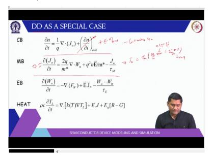
Now we can understand that drip division is a special case of this carrier valence and the momentum balance. So, the carrier balance if you recall if it is equilibrium dn by dt 0 plus you have generation term like electron hole pair generation. So, G - R due to electron generation mechanism. So, this is your basically carrier balance give you the continuity equation, it is a carrier continuity equation.
