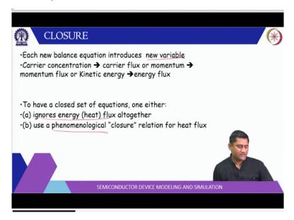
So, that means if you see all these three equations the equation for the carrier introduce J. So, in equation for carrier balance equation then we have the momentum balance equation. So, J it enters the W, then we have energy balance equation W which introduce the derivative of this F, the flux of energy density. So, the flux of carrier is current density, flux of current densities energy density and flux of energy and so on.
