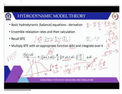
We will drive them from the Boltzmann transport equation. So, let us consider let us recall the Boltzmann transport equation where f is the distribution function. So, that means it tells you the number of electron or carriers with position r movement wave vector k at k 1 time t. So, it tells you the probability of finding electron at position r wave vector k at k 1 time t and of course if you integrate this distribution function you will get the number of carriers.
