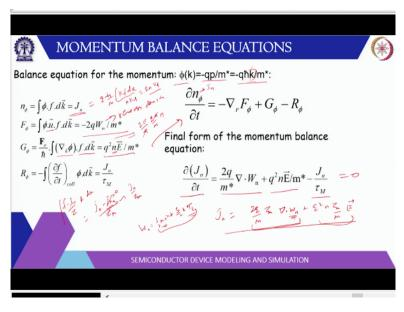
Now if we assume that phi is 1 then this n phi f phi G phi and r phi, this term simplify. So, this becomes integral f dk which is basically carrier consultation. So, left term becomes d n by d t. Then flux vacancy u f dk. Now u is the velocity f dk. So, f dk you can set is d n. So, it is like u dn. So, that will give you n times the average velocity or the drift velocity and which is basically related to the current density because j = q n v d.
