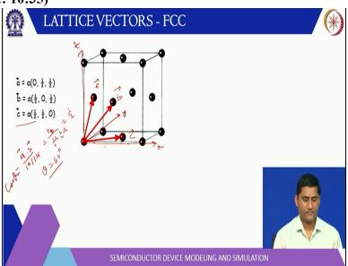
Similarly, we can calculate the lattice vector for FCC. So, for FCC, the 3 the nearest neighbor of the for this corner element, nearest neighbours of the face centers, so, this is the bottom face, this is the front face, this is the left face. So, the vector connecting the bottom phase, let us say this is x axis, this is y axis and this is z axis. So, bottom face will be a by  $2 \times x + a$  by
