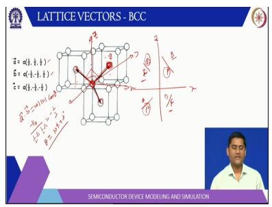
For a BCC now, you notice here is not a long x y z this lattice vector connects the nearest atoms. So, in a BCC it is a body's atom or the atom in the center at the center of the body which is nearest to the atoms as the edges. So, if you put let us 3 units cell together, so and connect this corner atom to body element of 1 body element of 2 and body element of 3. So, of course, first one will be this is let us say x this is let us say y and this is let us say this is z.
