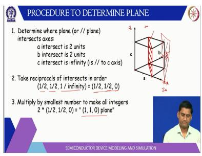
Now, how to determine the plane? So, if a given plan is given how do we name it? So, the standard procedure for naming the plane is first we find what are the intersects do to that plane on the x axis and y axis. Now, 2 planes if they are parallel and they can be said they are you know same plane basically except in certain situation. So, you can choose the origin nearby and then find the intersect.
