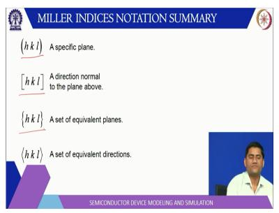
So, in summary we have discussed the miller indices notation we represent a plane by a simple bracket we represent a direction by a rectangular bracket we represent equivalent planes by curly brackets and we represent a set of equivalent directions by triangular brackets.
