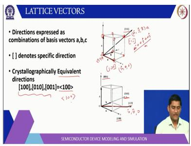
Now, let us vectors these are basically the vectors representing that direction in a semiconductor crystal. So, if you take let us say a simple cubic unit cell, there are 3 directions here a x axis y axis and z axis and simple cubic the atoms are at the corners here corners of the cube. So, if you consider the nearest atom now remember the lattice vector is drawn between or it is aligned connecting to nearest neighbours.
