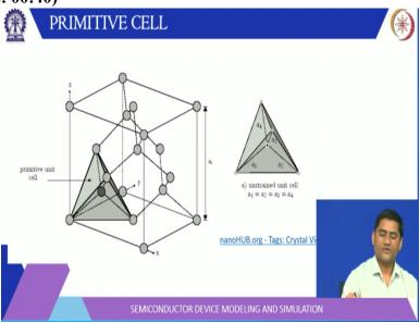
Last class, we discussed about unit cell structures. So, we discussed our simple cubic face centered cubic, body centered cubic diamond lattice. So, all these are lattice structures now, please remember the unit cell and the primitive unit cell they may not be same. So, for example, for diamond structure diamond lattice the unit cell is FCC, but the primitive unit cell is shown here certain data handling structure with the center there is 1 atom and followed by at 4 corners.
