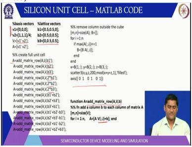
Here is one simple program which you can write in MATLAB. So, this is for silicone or diamond lattice so, here we define with this basis vector v1 and v2. Now, these are 2 items which form the basis. So, one is at 0 0 0 other is at A by 4 A by 4 A by 4. So, here we have taken equal to 1 because it is for representation purpose so, these to form the basis. So, now basis vector can be written as a combination of these 2 positions. Now, these 2 vectors can be combined these will be 2 positions.
