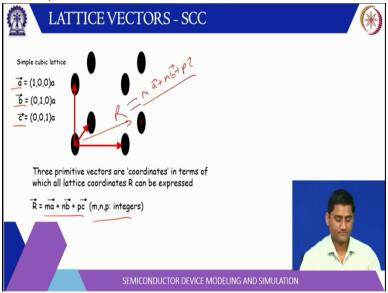
Now, we can find out the lattice vector for other cubic structures cubic cells, so of course in a simple cubic it is 1 0 0, 0 1 0 and 0 0 1 and many (())(05:11) of course, now, idea is that any lattice side any lattice point can be represented in terms of origin a distance is let us say R. So, R can be represented as a combination of these 3 primary or primitive vectors with some integer so, m is an integer times a, n is an integer times b plus p is integer times c.
