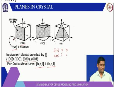
Now, once we know the lattice vectors, we can also describe the lattice planes in the crystal. So, a lattice plane is designated by the direction perpendicular to it. So, if the direction perpendicular to a plane is let us say 1 0 0 then the plane will also recall 1 0 0 the difference in the notation will be direction is represented by a square bracket and plan is represented by simple brackets and of course, similar to the equivalent direction which were represented by triangular brackets.
