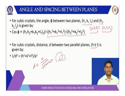
Now, for the cubic crystal, the angle between 2 planes is same as the angle between the perpendicular directions of those planes. So, let us say you have h 1 k 1 l 1 is 1 plane h 2 k 2 l 2 is another plane. So, corresponding direction will be h1 k1 l1, h2 k2 l2. So, if you want the angle between 2 vectors again a dot b is ab cosine phi. So, cosine phi will be a dot b, a dot b h1 h 2 + k 1 k 2 + l 1 l 2 divided by magnitude of individual vectors.
